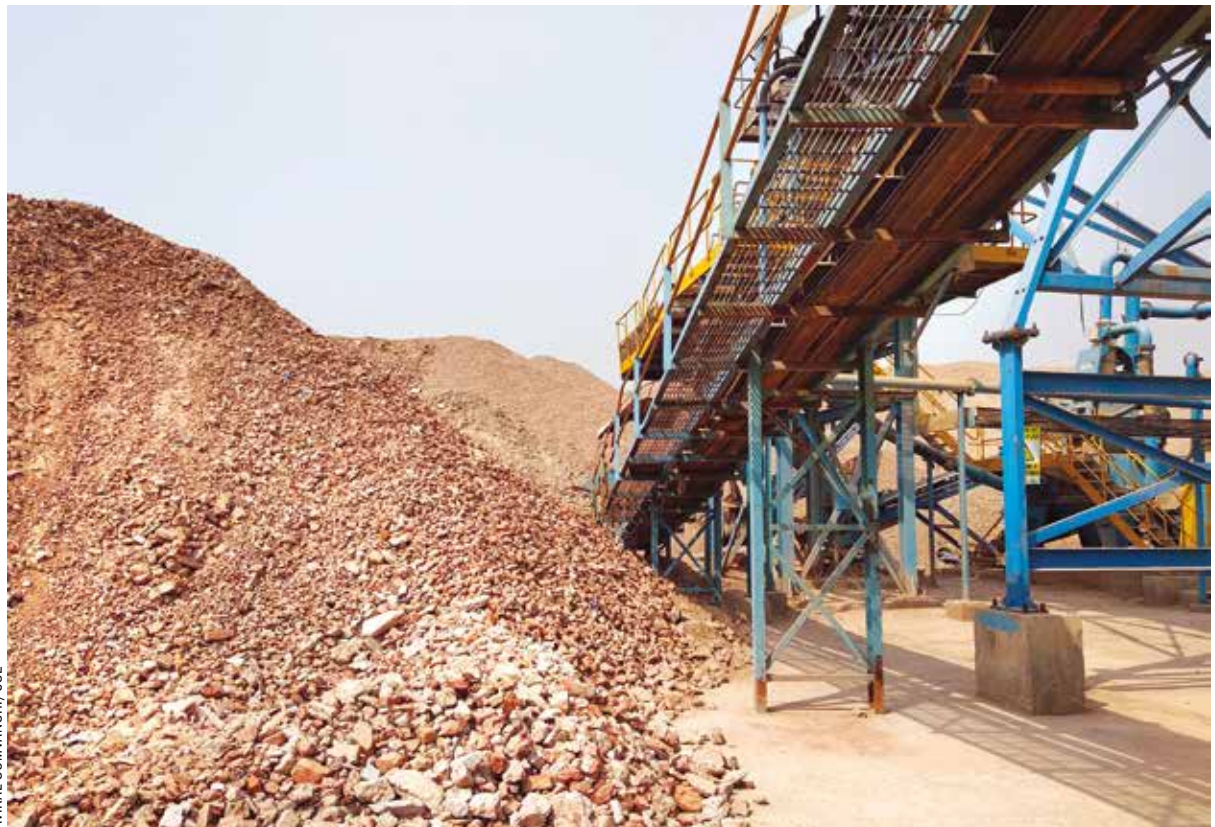
A pile of recycled aggregate manufactured from recycled C&D waste at Delhi's recycling facility
