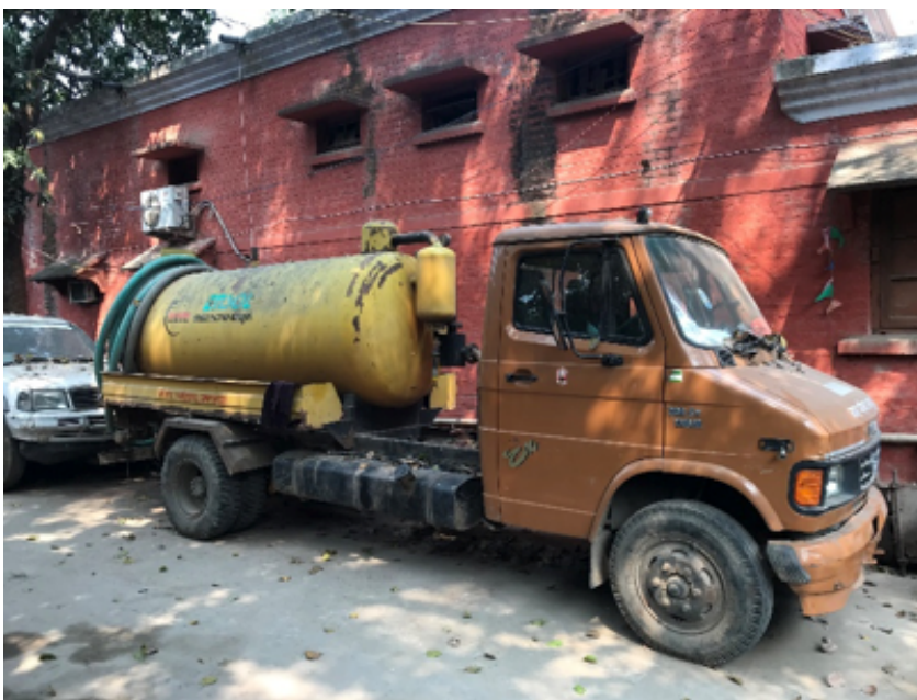
Truck mounted vacuum tanker, Jamalpur
