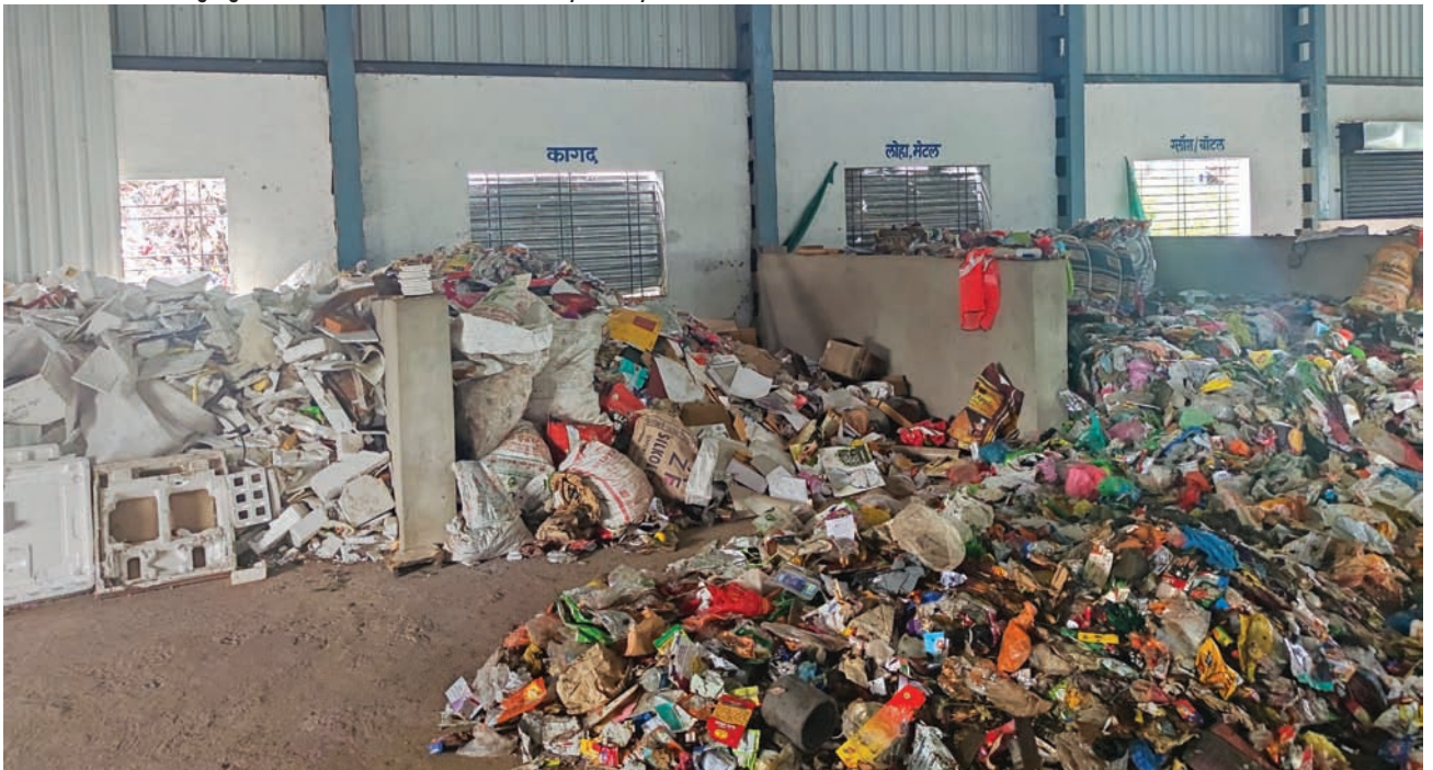
Sub-segregated waste at the material recovery facility
