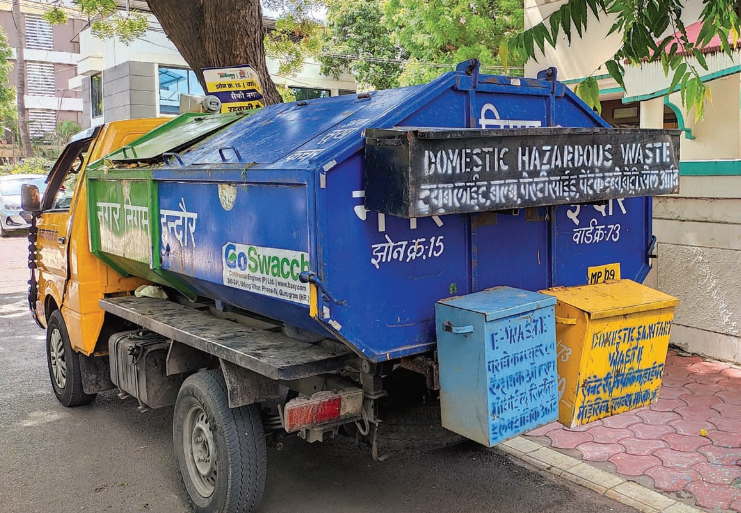
Compartmentalised vehicle for collection of biodegradable, non-biodegradable, domestic hazardous, electronic and sanitary wastes
