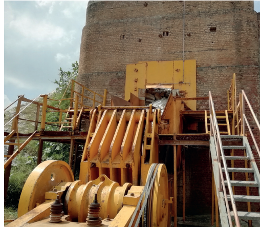
Unloading point for raw material (deep pit feeder)
