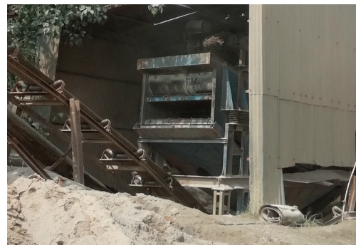
Photographs 16: Partially covered or damaged sheds for dust containment
