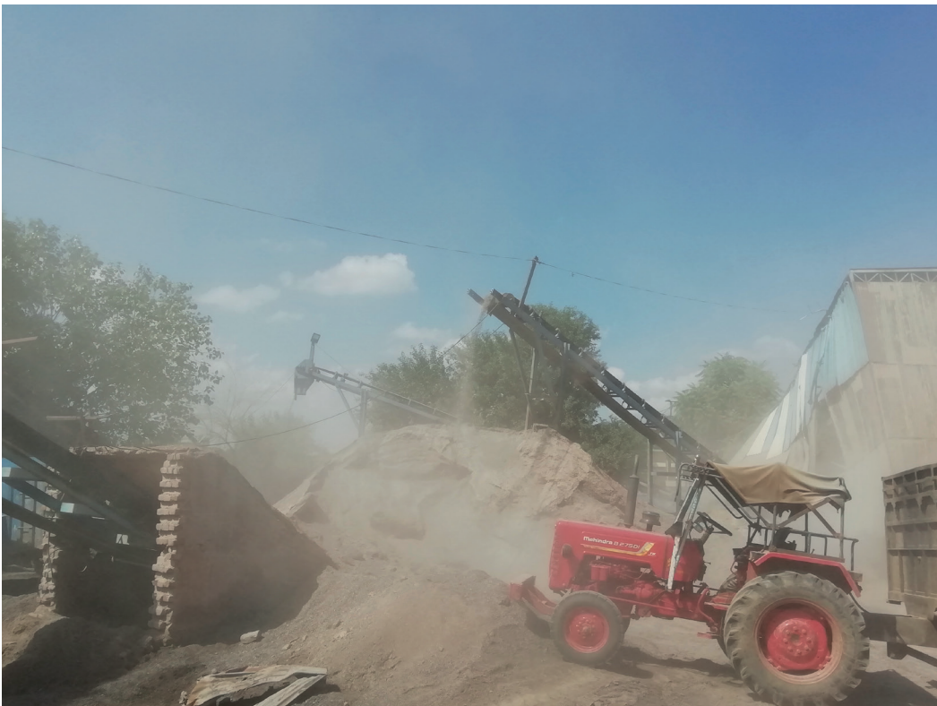
Fugitive emissions from operation of a stone-crusher unit
