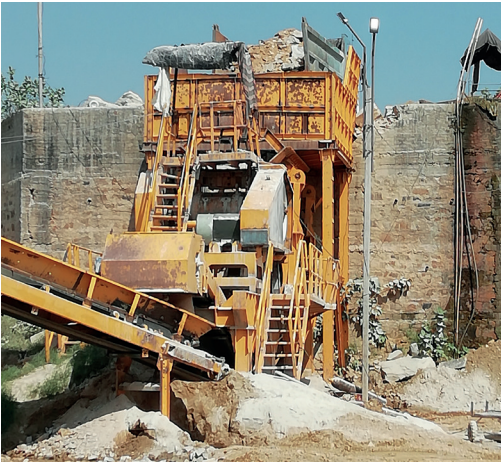
Jaw crusher with elevated feed hopper
