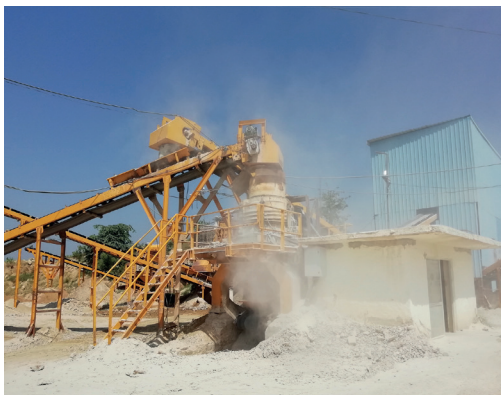
Photograph 10: Fugitive emissions from secondary crushing
