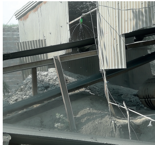
Water sprinklers provided on conveyor belts
