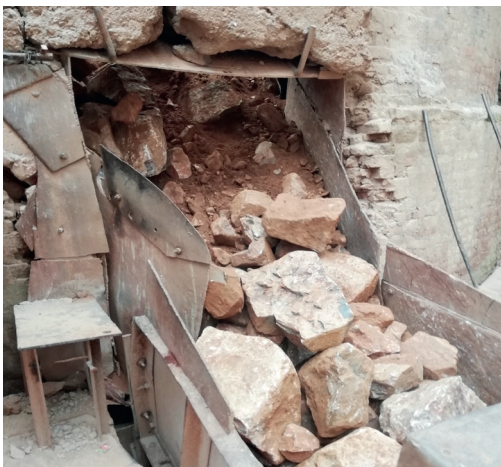
Raw material fed to jaw crusher from feeder
