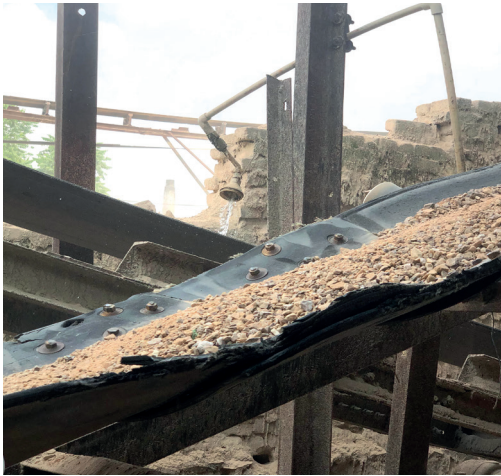
Water sprinklers provided on conveyor belts
