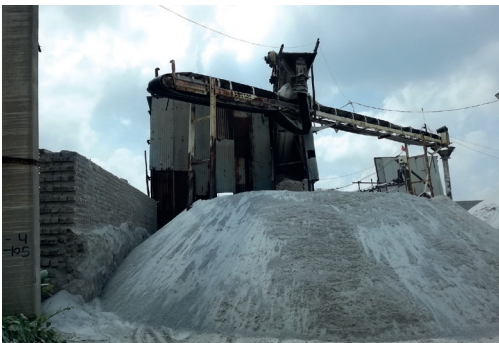
Inadequate height of wind-breaking wall
