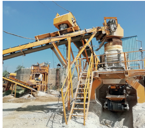
Cone crusher for secondary crushing
