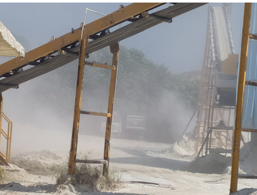
Photograph 15: Dust emissions during product release at stockpile
