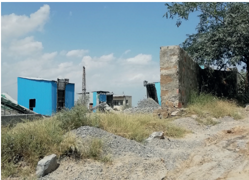
Inadequate height of boundary wall at stone-crushing units
