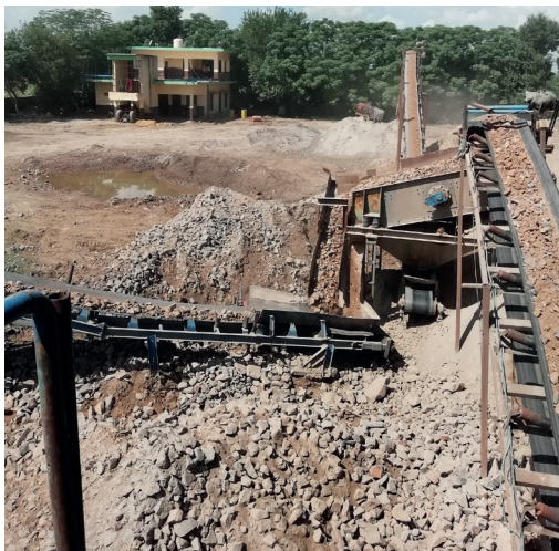
Conveyor belt system in a stone-crushing unit
