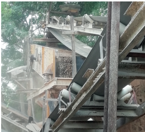
Photograph 12: Fugitive dust from screening process
