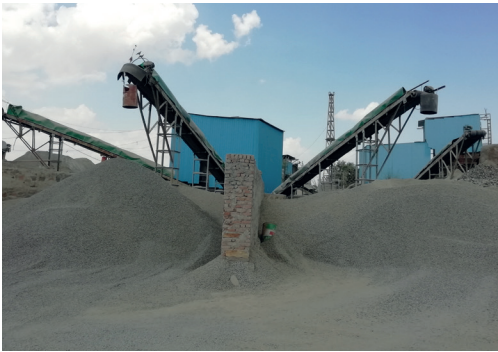
Inadequate height of wind-breaking wall
