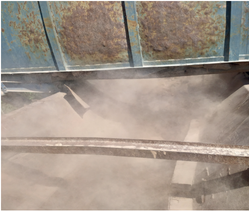
Photograph 8: Emissions from primary crushing
