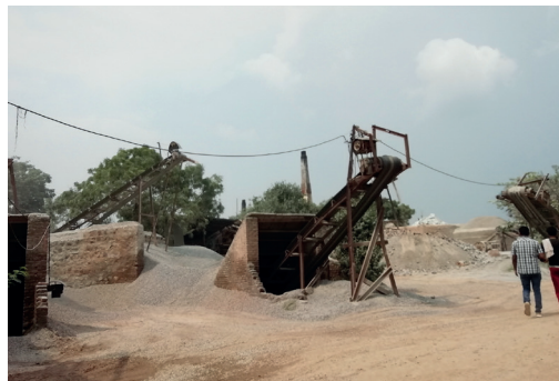
Inadequate height of wind-breaking wall
