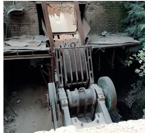
Raw material fed to jaw crusher from feeder
