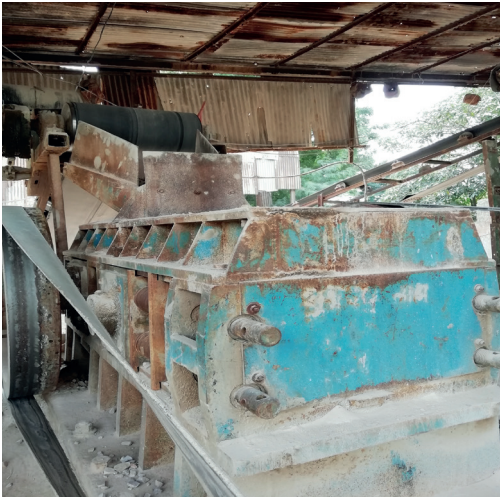
Photograph 5: Tertiary screening unit
