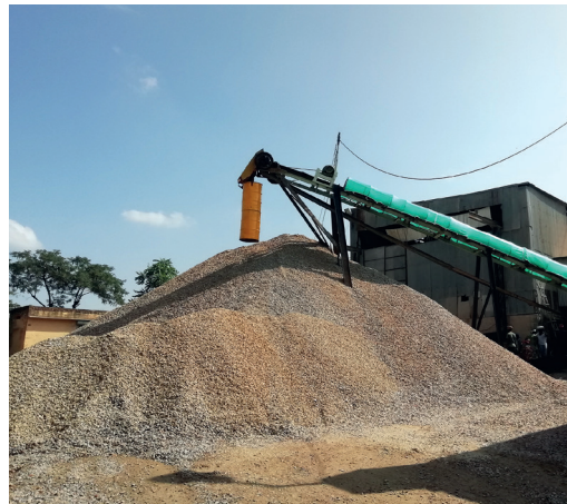
Chute for release of final product to stockpile
