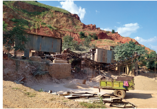
Inadequate height of wind-breaking wall
