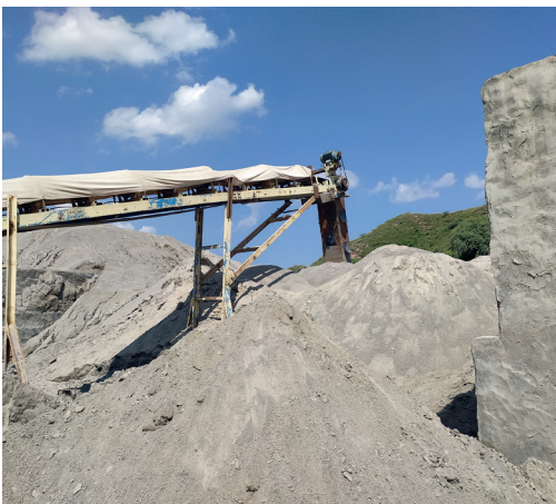
Chute for release of final product to stockpile
