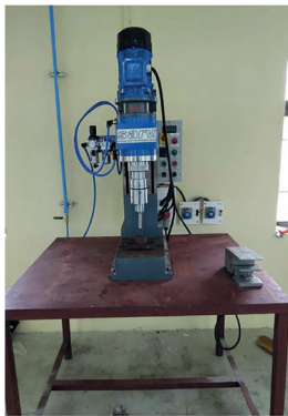
Image 13: Brake and clutch liner riveting machine
