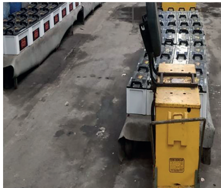
Image 33: Correct practice Battery is placed on a table while charging
