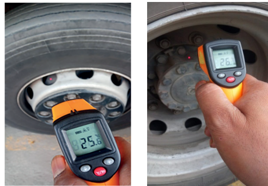
Image 40: Measuring wheel temperature
