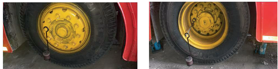
Image 41 and 42: Checking wheel free rotation of both front and rear wheel
