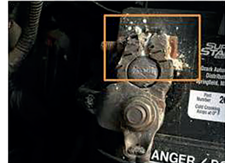
Figure 2: An unclean plug causes sulphation
