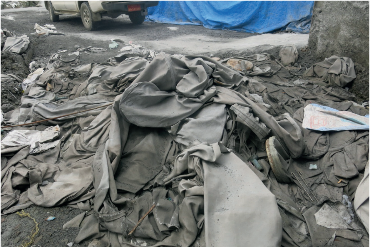
Figure 28: Discarded bag filters—no designated place for disposal
