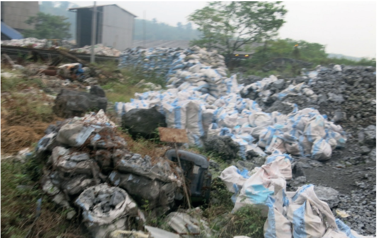
Figure 29: Raw material storage and handling not proper, it adds to the fugitive emission
