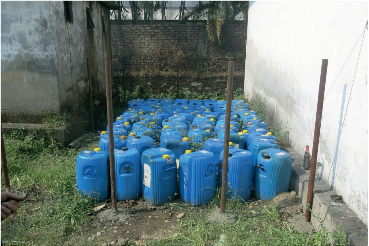
Figure 30: HCL stored in the open without any liner—high risk of soil and ground water contamination
