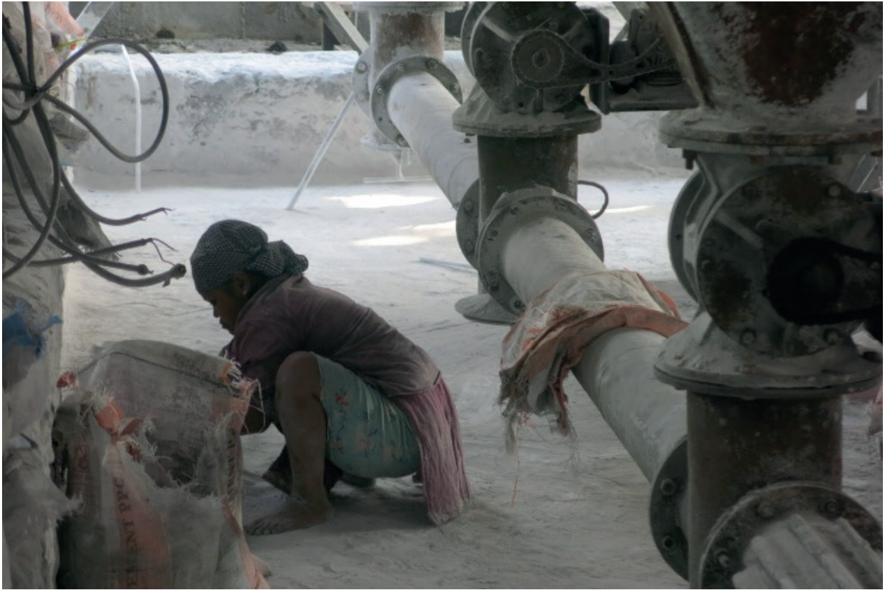
Figure 36: Manual dust collection in most of the industries
