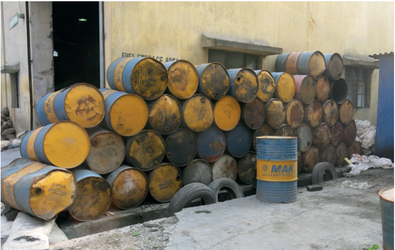
Figure 25: Storage of used oil drums near storm water drains — can lead to water contamination
