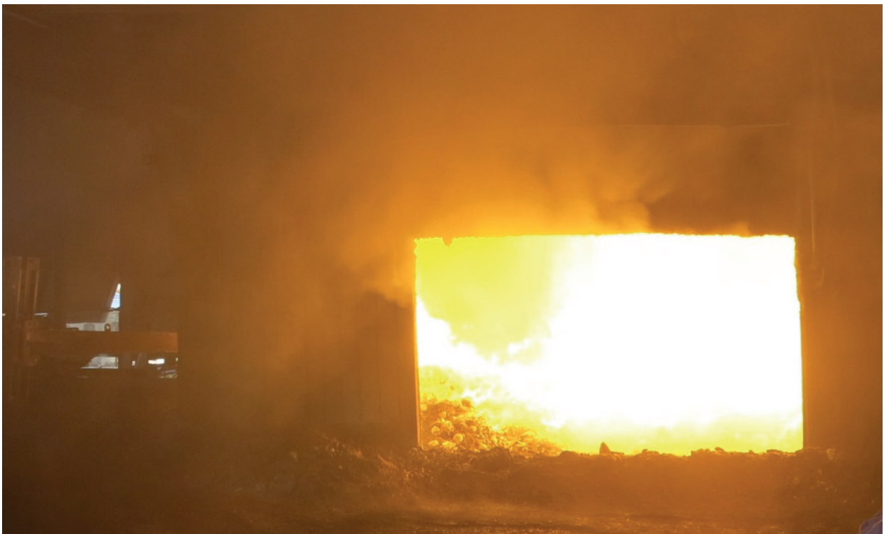
Figure 15: Fugitive emission from open furnace due to inappropriate functioning of fume extraction system
