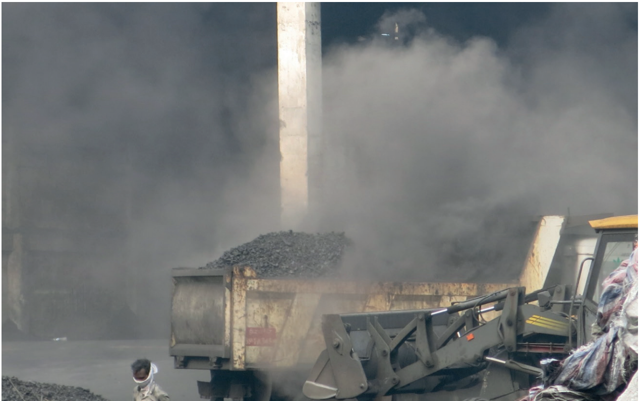
Figure 21: Poor road condition in the area adds to the fugitive emission during transportation of raw material
