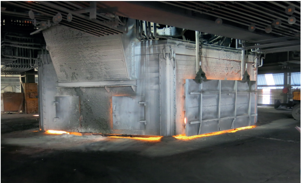
Figure 17: Hydraulically operated furnace doors to control fugitive emission—Reduces fugitive emission
