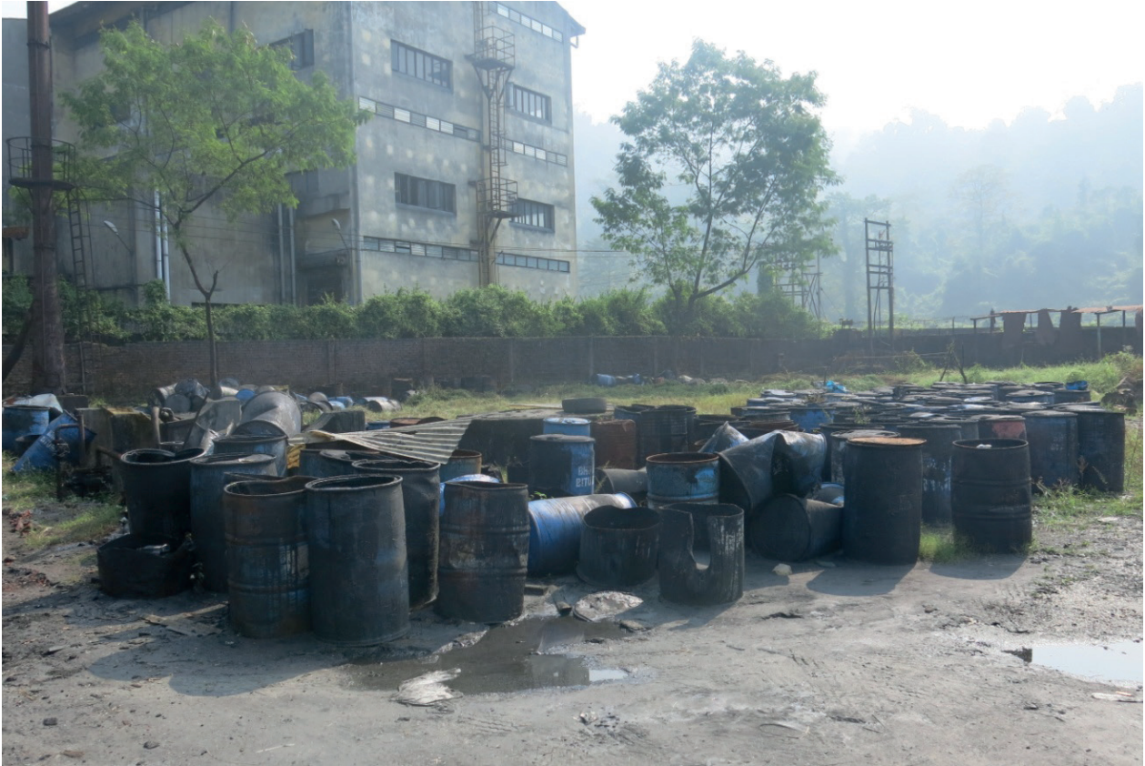
Figure 24: Bhutan Bitumen poor housekeeping —no designated place for storage
