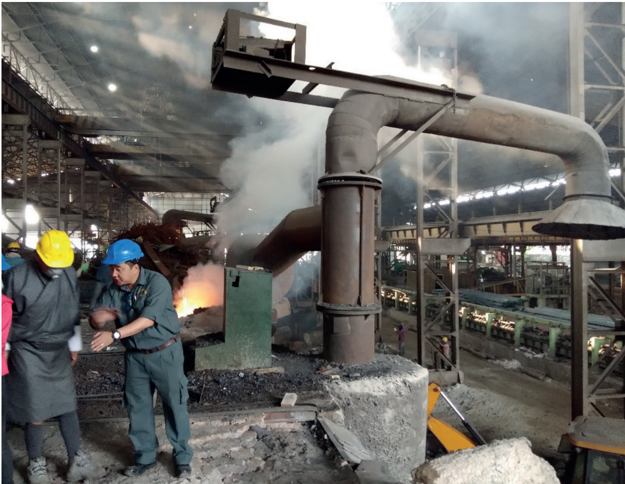
Figure 11: Ineffective fume extraction at Lhaki Steel
