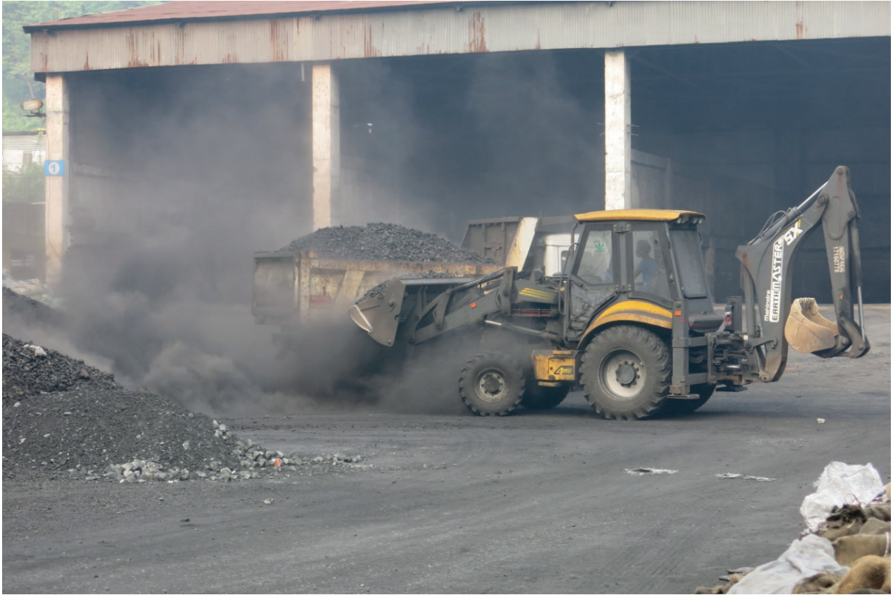
Figure 19: Fugitive emission during loading and unloading of material—most industries store raw materials in open
