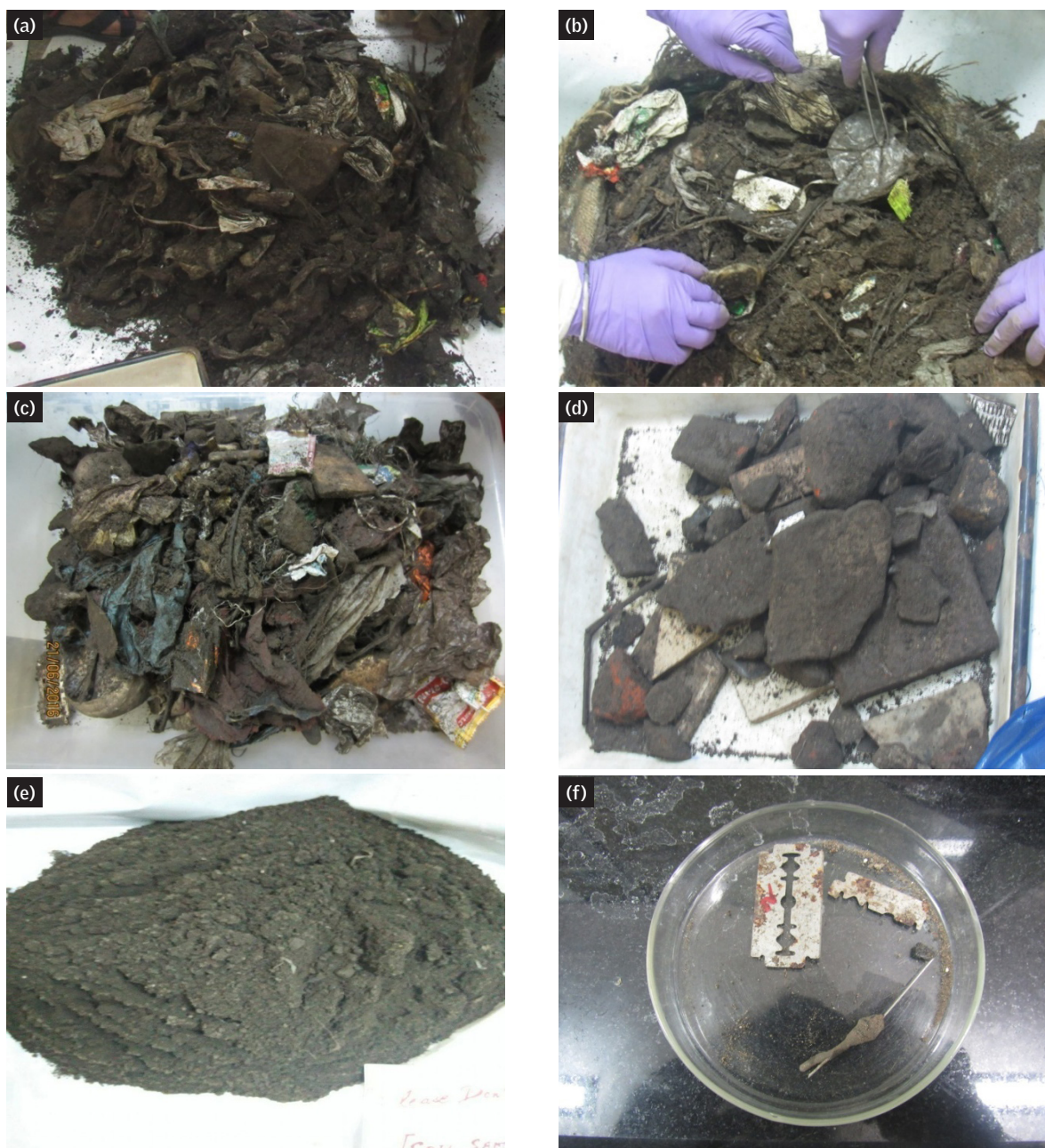
Various fractions of legacy waste obtained after sampling and segregation of waste from the Pirana dumpsite: (a) Mixed waste received at Pirana dumpsite in 2017; (b) Manual segregation of waste; (c) Scrap polymeric and combustible materials (d) Inert waste of size >10 mm; (e) Fine fraction of size <6 mm; (f) Miscellaneous items like razors and needles
