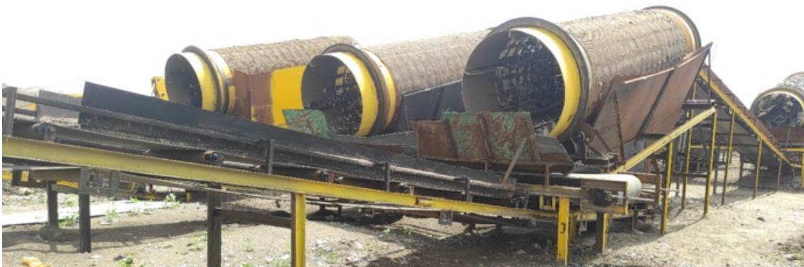
Trommel screens used in legacy waste size segregation
