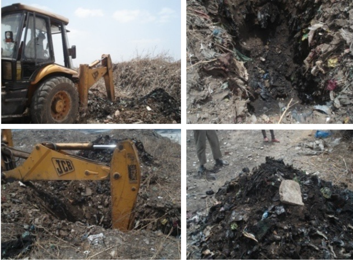
Typical sampling of legacy waste using a JCB—Pirana dumpsite Left (top and bottom): Front-hoe loaders used for legacy waste sample collection from the surface of the dumpsite Right (top and bottom): Legacy waste sample pit
