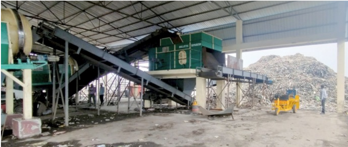
Ballistic separators used in legacy waste sorting
