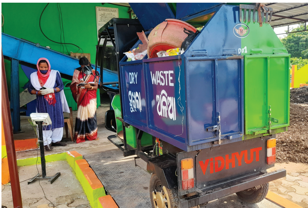
Door-to-door collection vehicles being weighed on a processing facility's weighbridge
