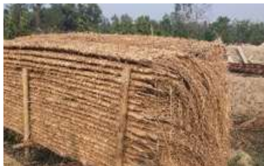
Thatch panels made of split bamboo and rice straw
