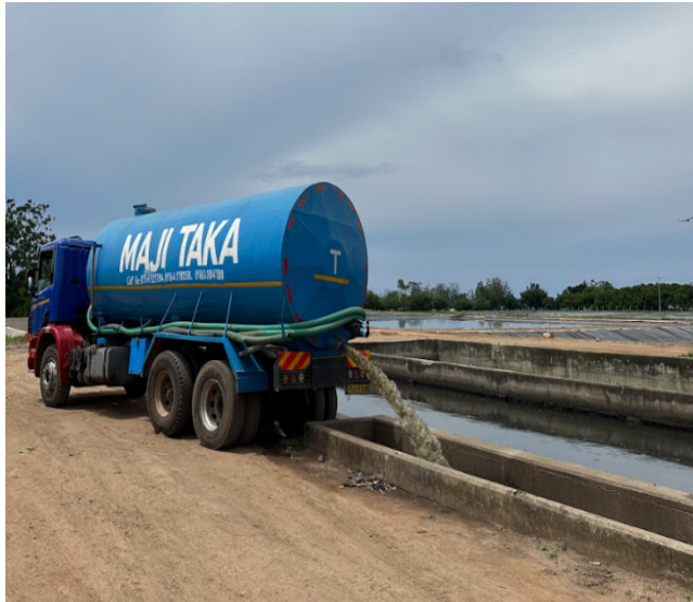
Private desludger decanting at the faecal sludge decanting point at the waste stabilization pond at Butuja
