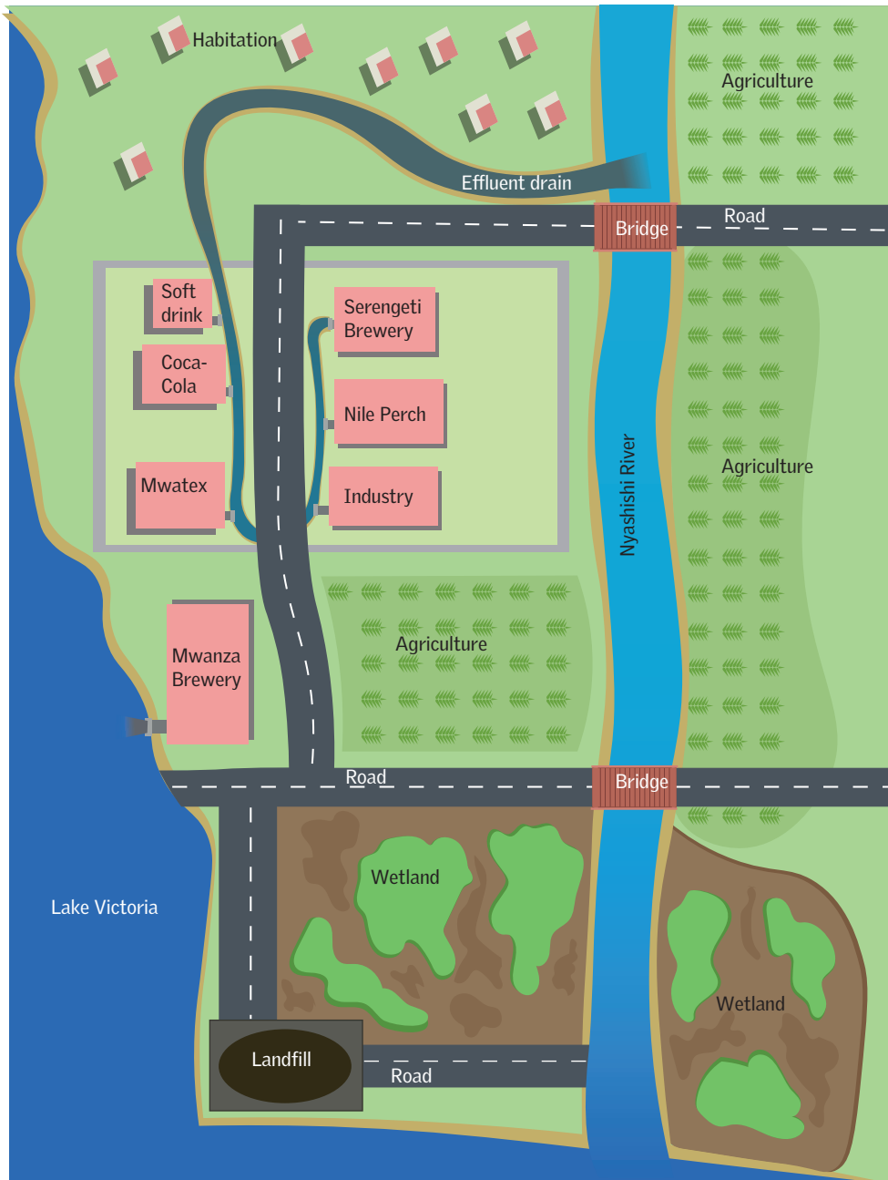
Figure 7: Schematic diagram of industrial wastewater discharge to the Nyashishi riverine system
