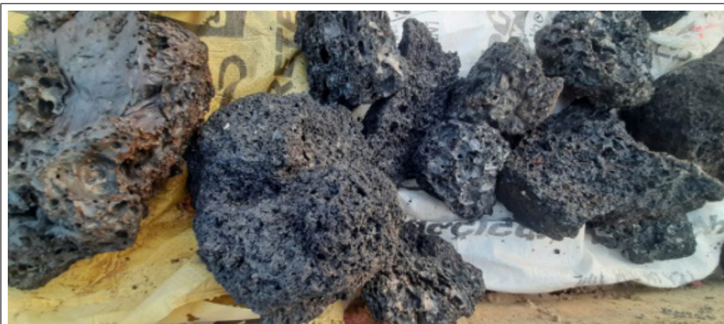
Photograph 11: Cinder materials used in the integrated settler and anaerobic filter (ISAF)
