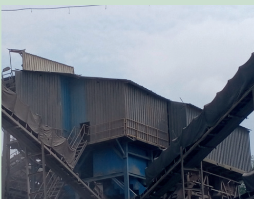
17d. Covered screen with door arrangements
