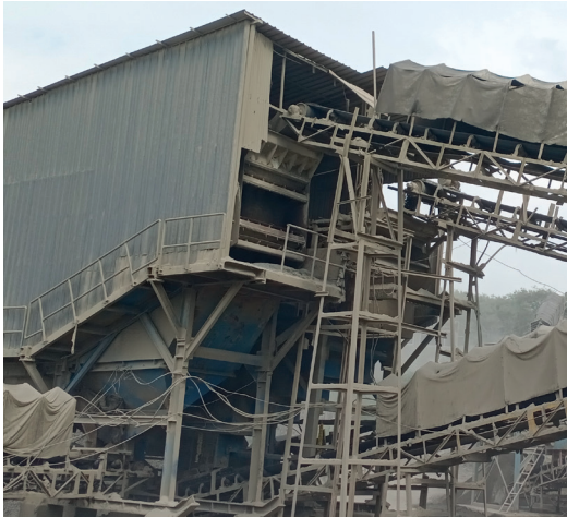
13a. Screen with door arrangement
