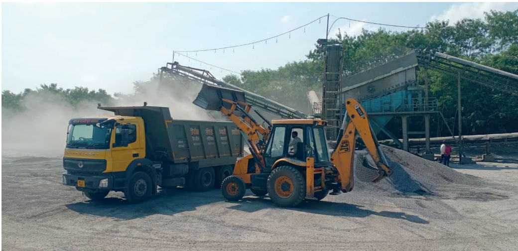
8b. Fugitive emissions generated at the time of loading of product
