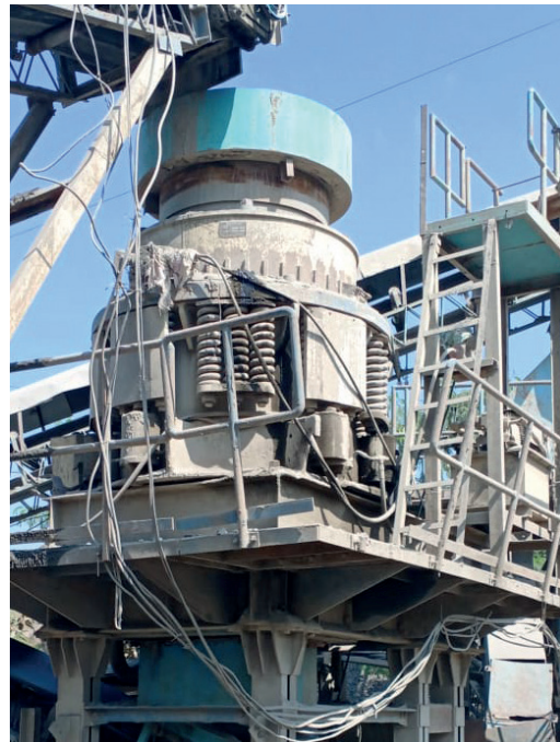
5b. Cone crusher for secondary crushing
