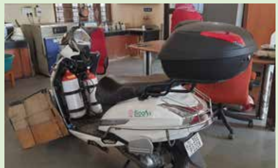
2-wheeler integrated with bio-CNG kit ▲
