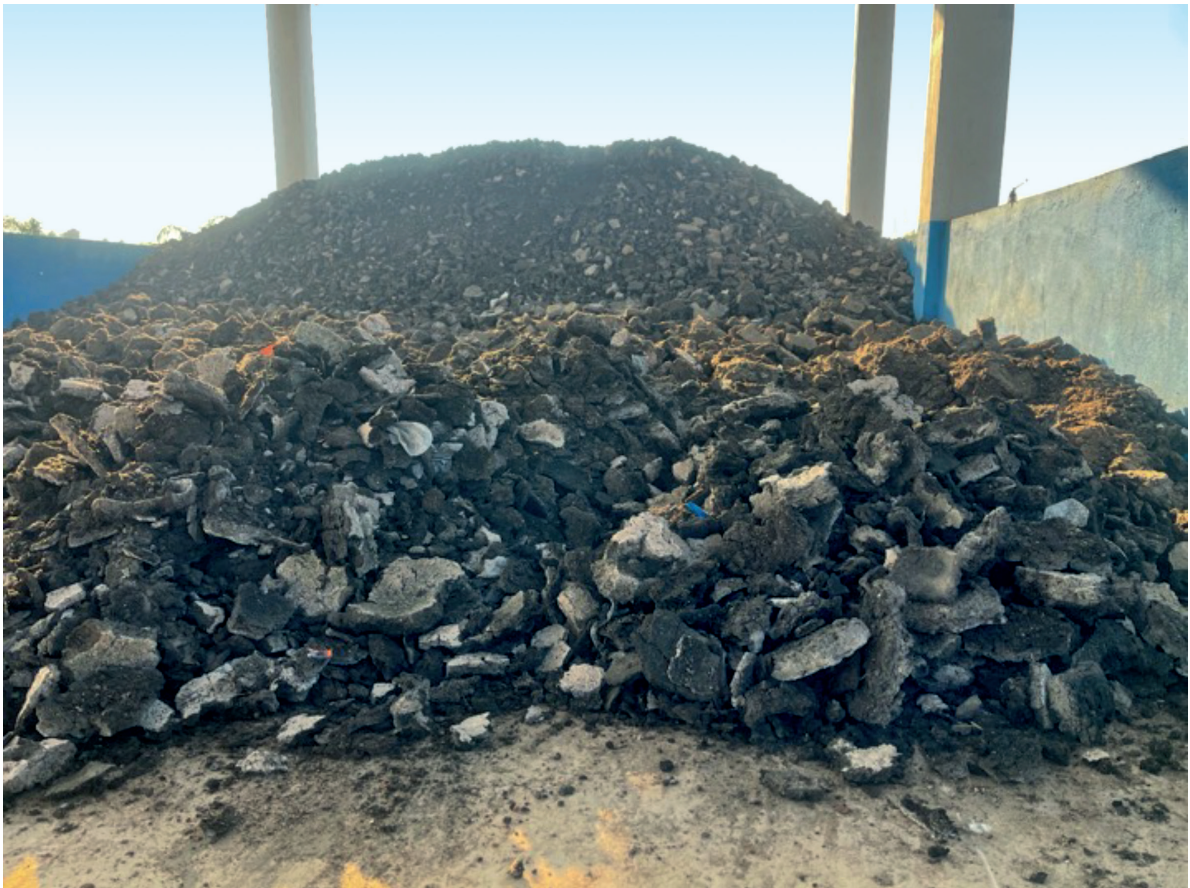
Storage of biosolids in the FSTP sites
