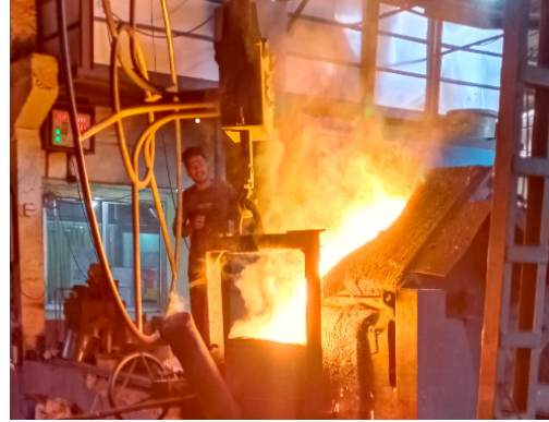
7b. Fugitive emissions at an induction furnace
