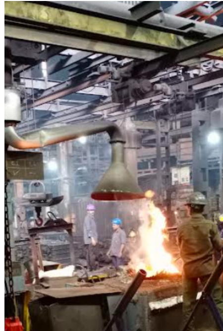
12b. Hood installed at the induction furnace
