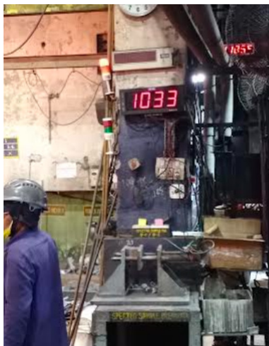
12c. Temperature sensor installed at the furnace
