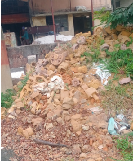
10a. Broken moulds dumped outside a foundry
