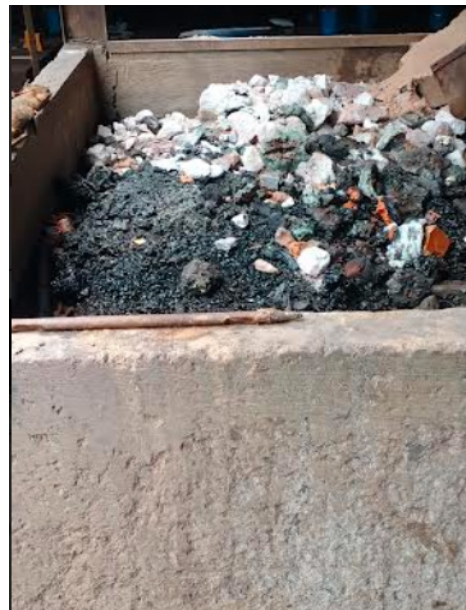
8b. Slag stored in a wet scrubber tank
