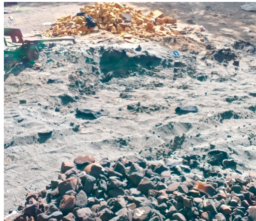
10f. Burnt sand dumped inside a foundry
