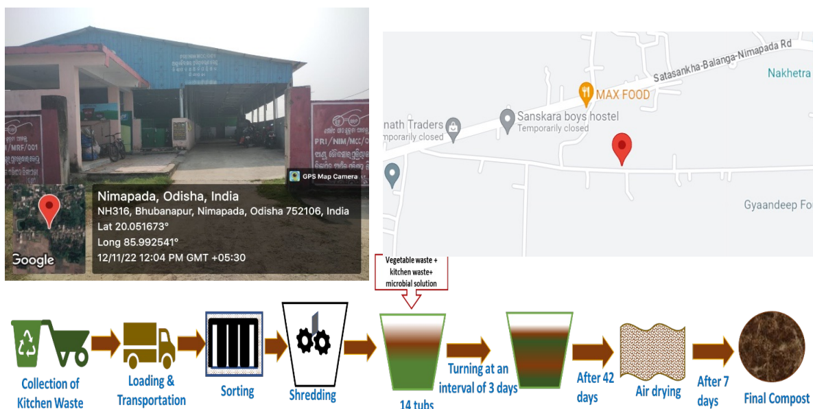
Picture 20: Location and flow diagram of composting unit in Nimapada
