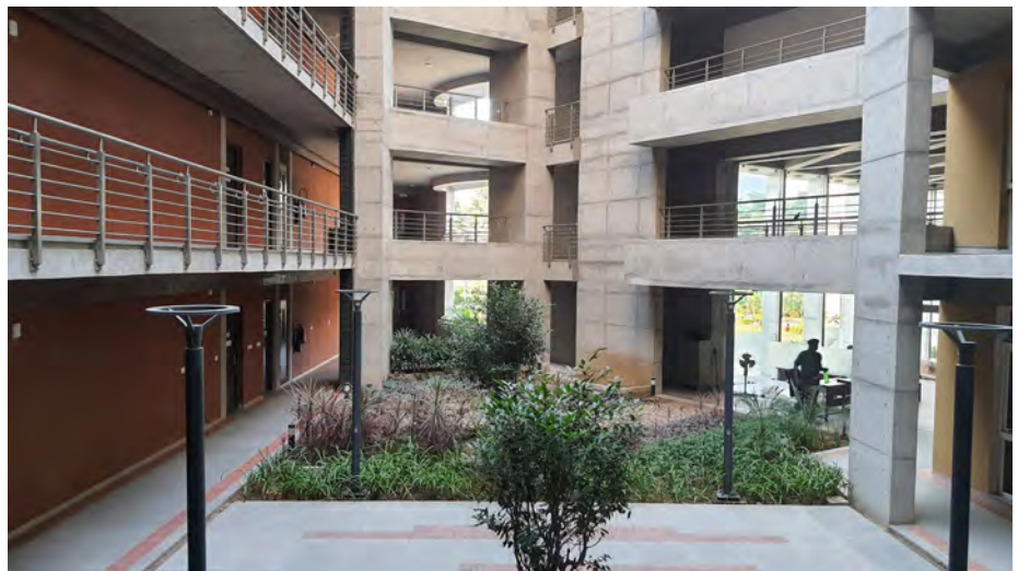
The narrow courtyard along with a pergola keeps the courtyard shaded while the evapotranspiration from the vegetation works to cool ambient air.
