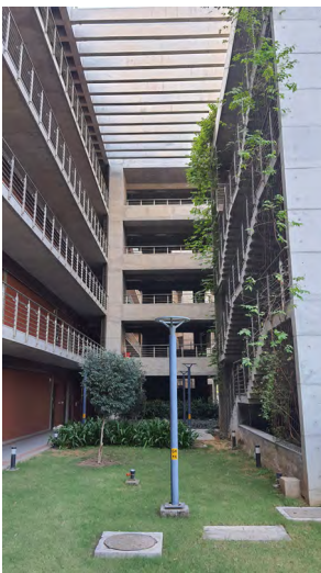
The narrow courtyard along with a pergola keeps the courtyard shaded while the evapotranspiration from the vegetation works to cool ambient air.
