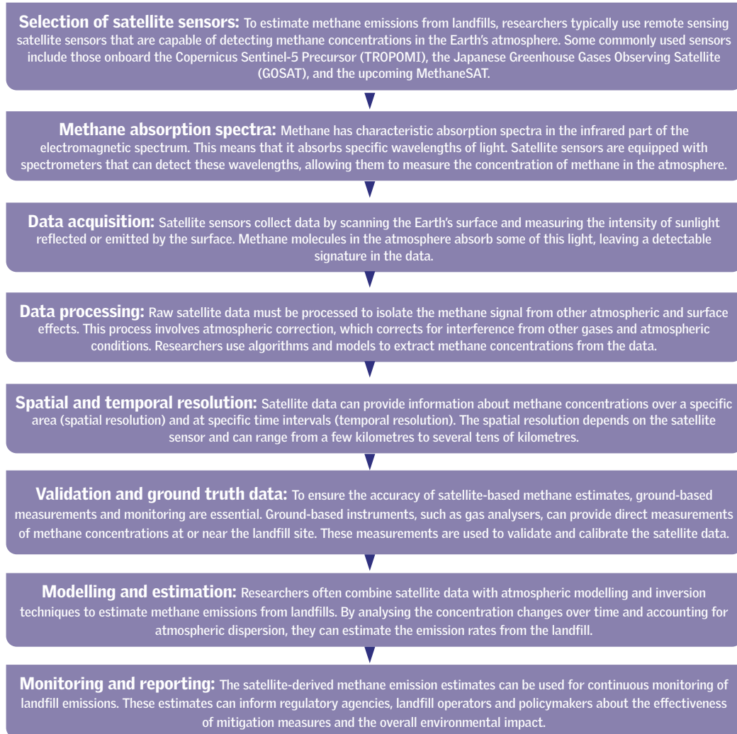
Figure 5: Various steps involved in methane estimation by satellites
