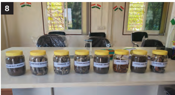
7. Processed aggregate stored on site; 8. Different types of processed re-usable aggregates
