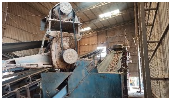
Interior of a Dry Processing Unit: Conveyor belts moving different sized particles after screening
