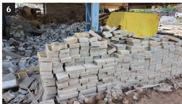
5. Aggregates of different size are received after processing; 6. Moulds for making pavers; 7&8. Recycled products
