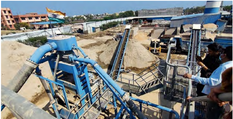
Filter/screen for separation (left); cyclone jumper machine (right)
