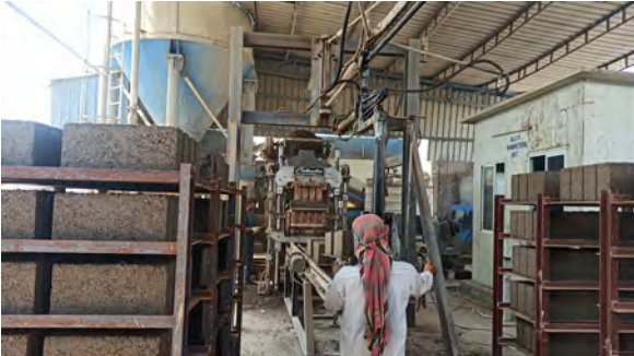
Block making process: Pressing machine (left) and storing to rack (right)
