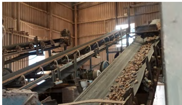
Interior of a Dry Processing Unit: Conveyor belts moving different sized particles after screening
