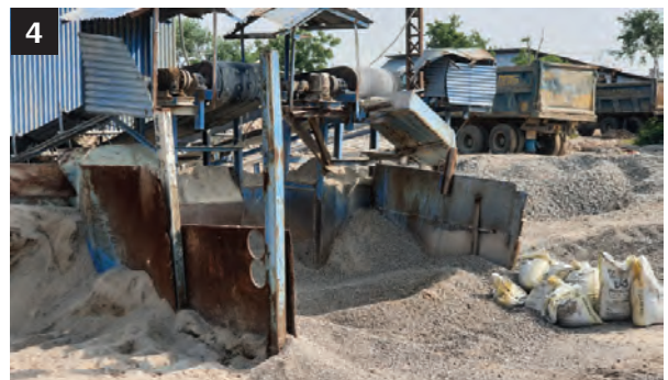
1. Weighing bridge at Burari C&D waste recycling plant; 2. Segregation of inerts; 3. C&D waste processing unit at Burari C&D waste recycling plant; 4. Aggregates of different size are received after processing
