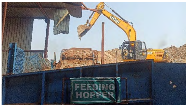
Waste being fed into the feeding hopper (left) Manual segregation (right)
