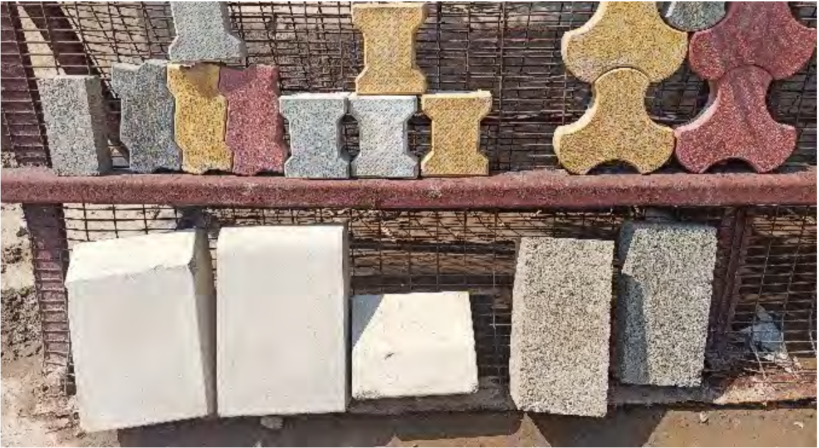
The plant produces zigzag, dumbbell-shaped and Milano tiles (top, left to right), kerbstones (bottom left) and concrete blocks (bottom right)
