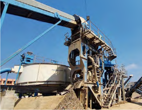
Dewatering screen for removal of light materials
