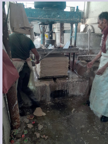
Pressing for dewatering
