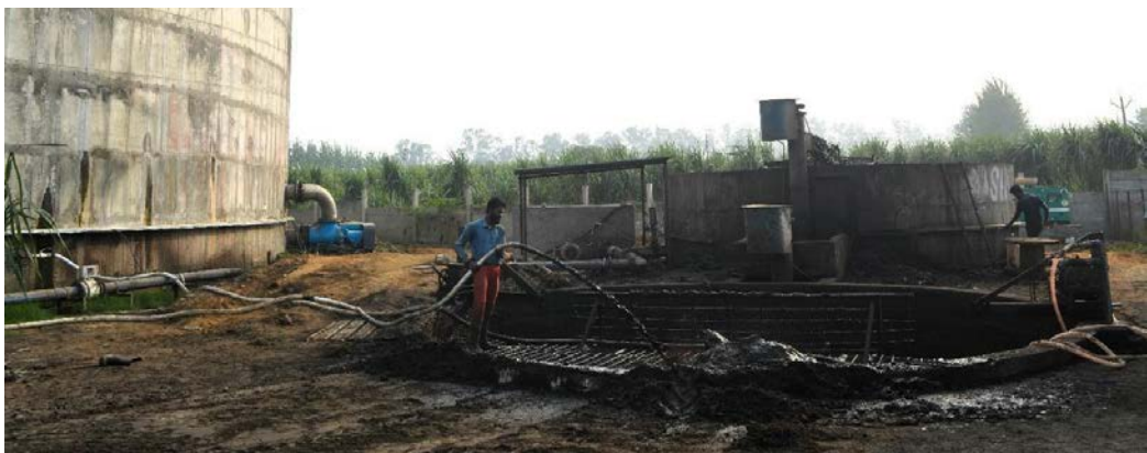
Image 7: The water being mixed with the feedstock in the mixing tank to be fed into the bioreactor
