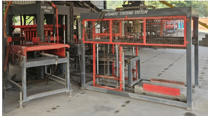
Image 43: Brick/Block manufacturing machine at the Chandigarh plant
