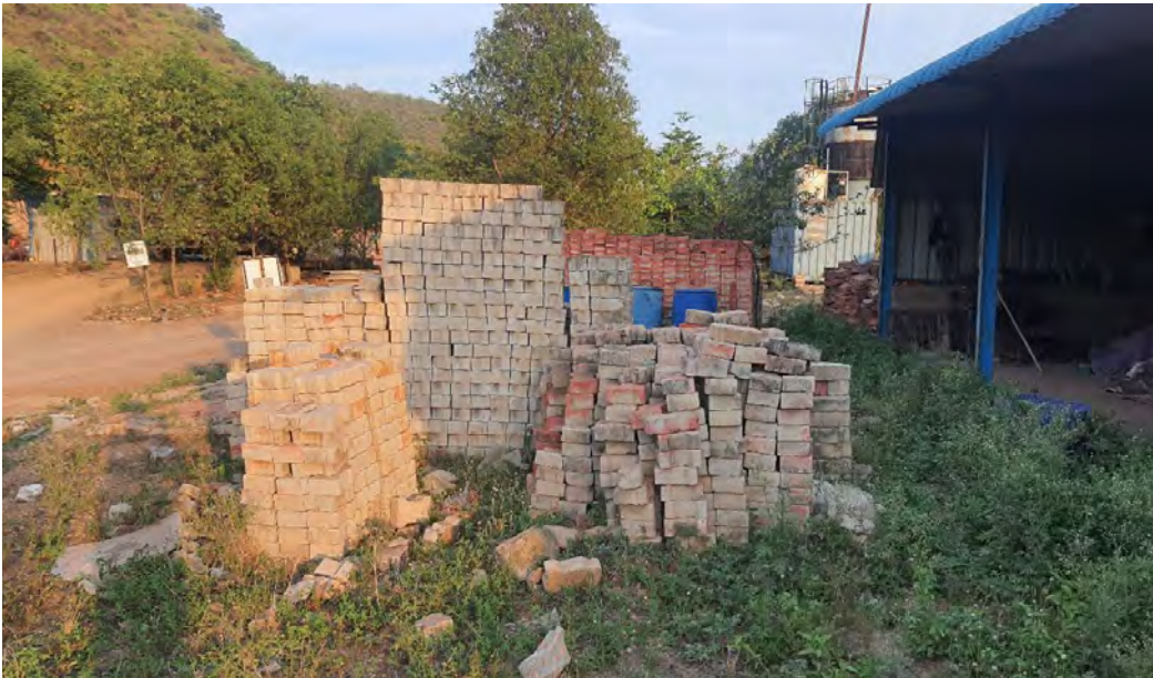
Image 49: Paver blocks of various sizes and shapes at Vishakapatnam C&D recycling plant
