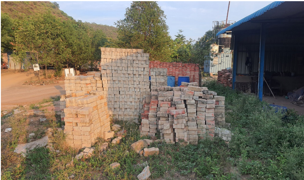
Image 49: Paver blocks of various sizes and shapes at Vishakapatnam C&D recycling plant
