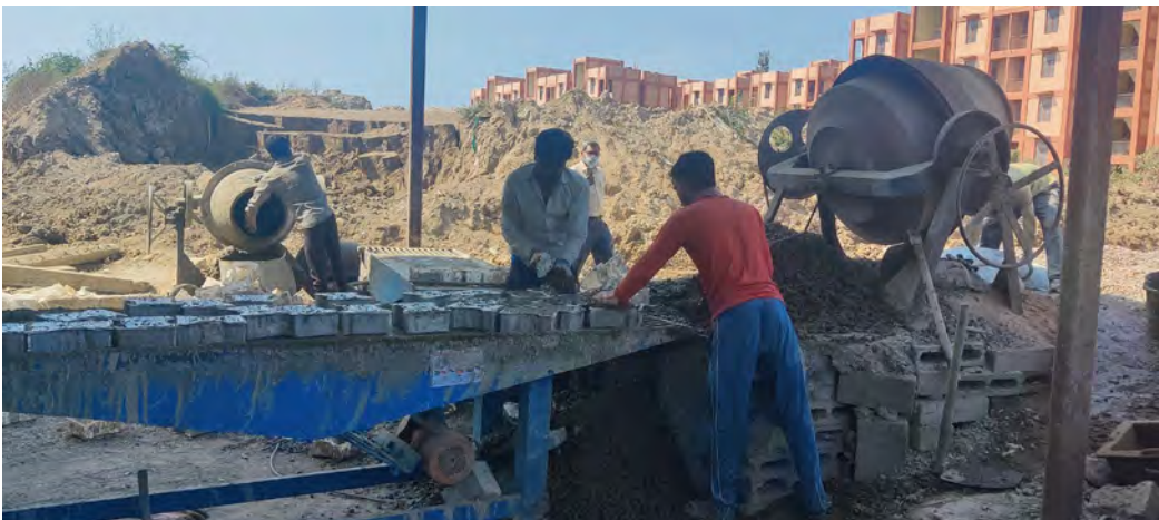
Image 41: Tiles being manufactured with the help of plastic moulds, Bakkarwala, Delhi
