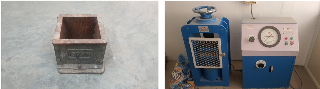
Image 59-60: Apparatus for carrying out concrete cube test at Jeedimetla plant, Hyderabad
