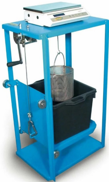
Images 56 and 57: Apparatus used in water absorption test
