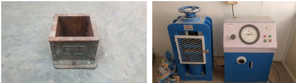
Image 59-60: Apparatus for carrying out concrete cube test at Jeedimetla plant, Hyderabad
