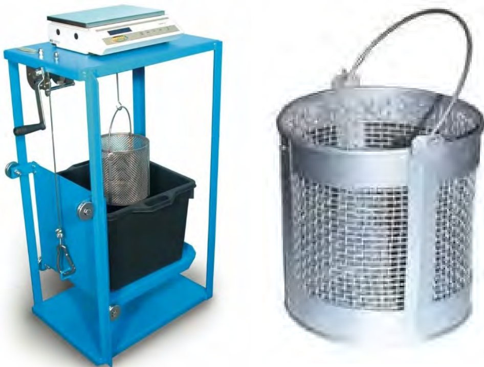
Images 56 and 57: Apparatus used in water absorption test
