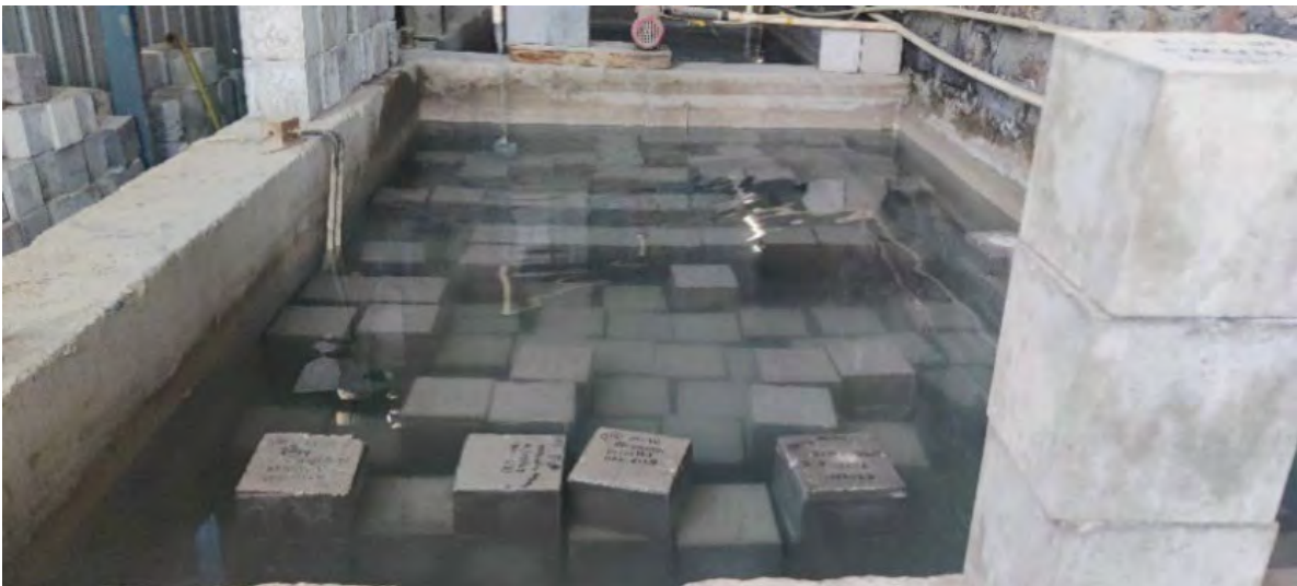
Image 61: Curing of concrete cubes taking place at the Bakkarwala plant, Delhi
