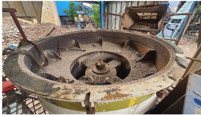
Image 26: Vertical Shaft Impactor at Fathulaguda plant, Hyderabad
