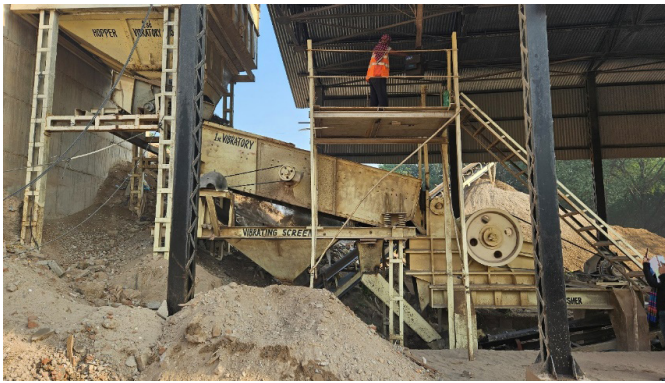
Image 22: Grizzly screen at Chandigarh C&D recycling plant
