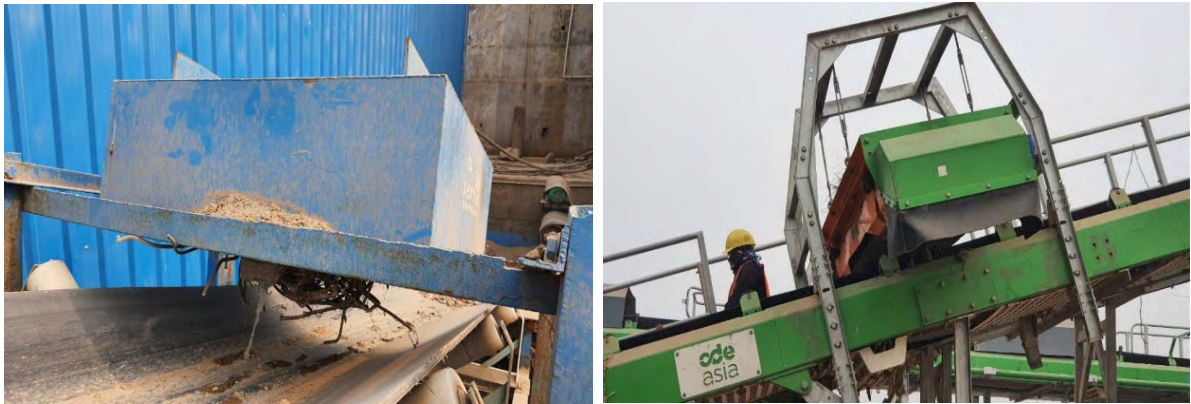
Image 28: Overhang magnetic separator installed at Greater Noida (Left) and Over band magnetic separator in Burari, Delhi (Right)
