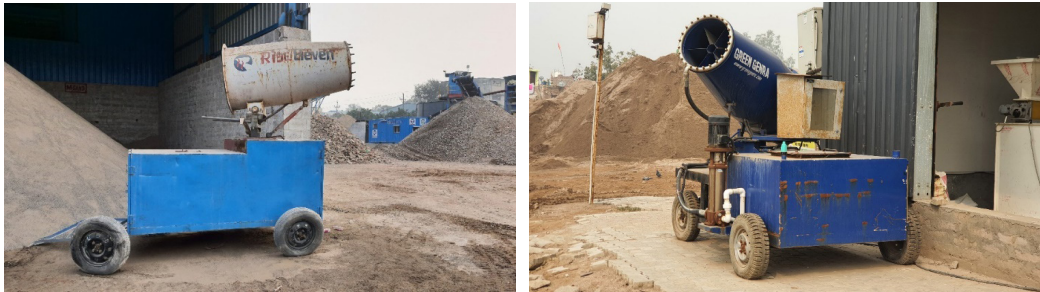
Image 36: Anti-smog gun at Greater Noida plant and Burari, Delhi
