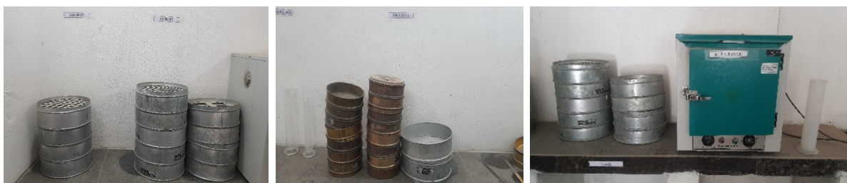
Images 53-55: Sieve analysis equipment at the Jeedimetla C&D recycling plant in Hyderabad
