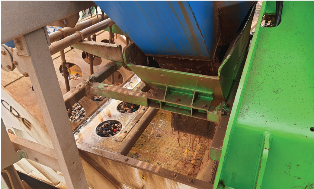
Image 30: Wood and other lightweight plastics getting separated in a log washer in Burari, Delhi
