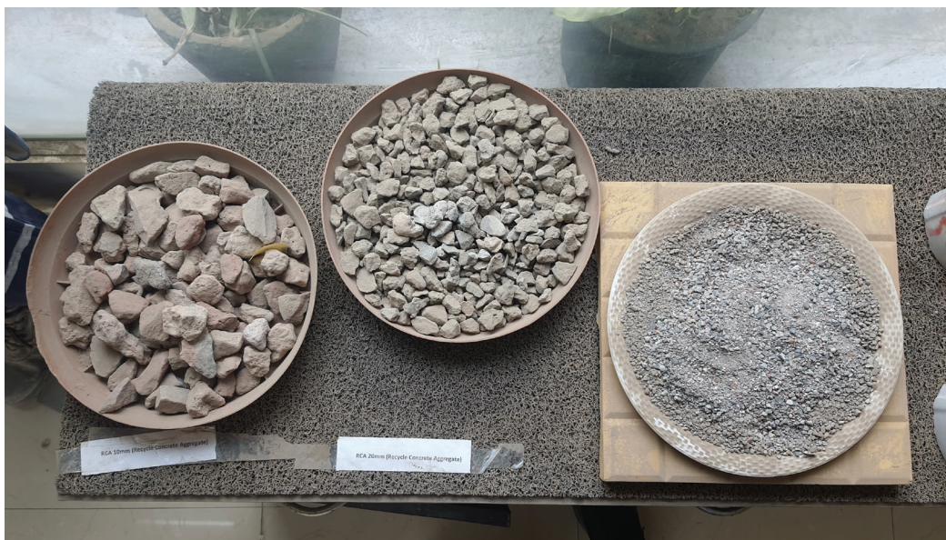
Image 44: Recycled aggregates (Left) Recycled concrete aggregates (Centre) and Sand (Right) at Burari plant, Delhi
