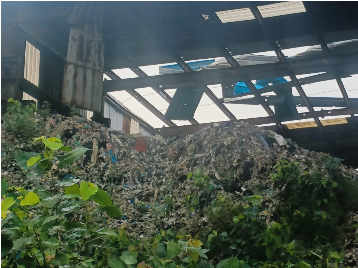
SCF recovered from biomining of Kuberpur site temporarily stored in a storage shed
