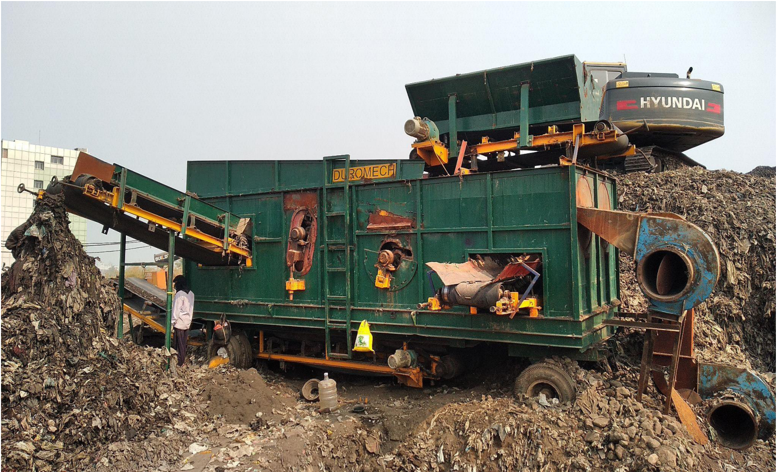
Air density classifier (ADS) for segregation of SCFs from biomining of legacy waste
