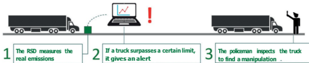
Figure 4: Real driving emission monitoring for heavy duty vehicle to catch AdBlue killers
