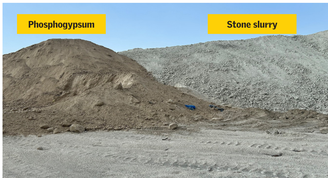
Industrial waste—Phosphogypsum and stone slurry used as a raw material for making gypsum
