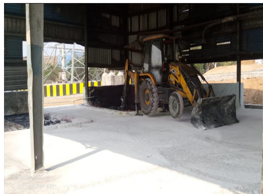
Preparation of AFR by mechanical mixing
