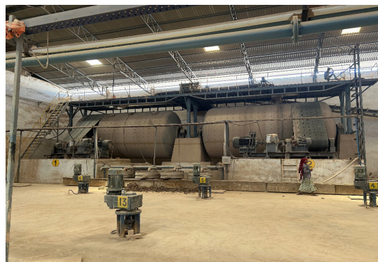
Mixing of raw material in ball mill
