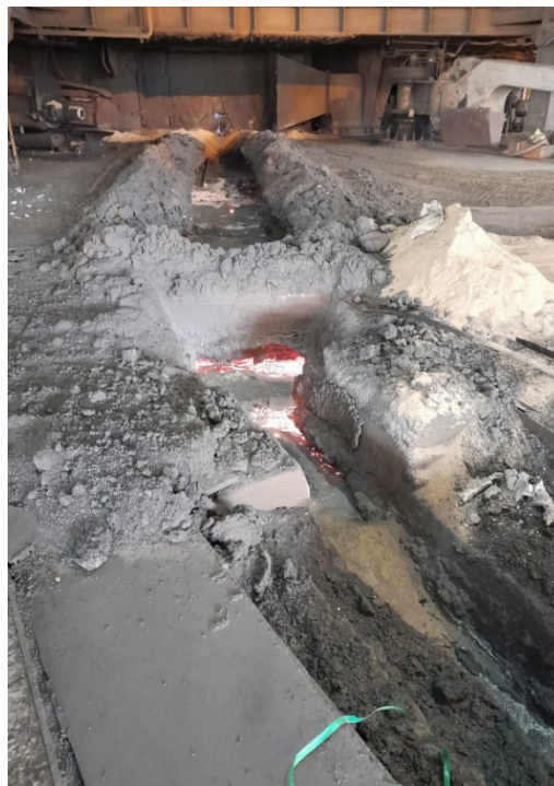
Trenches to extract hot metal from blast furnace and use of slag as runner material
