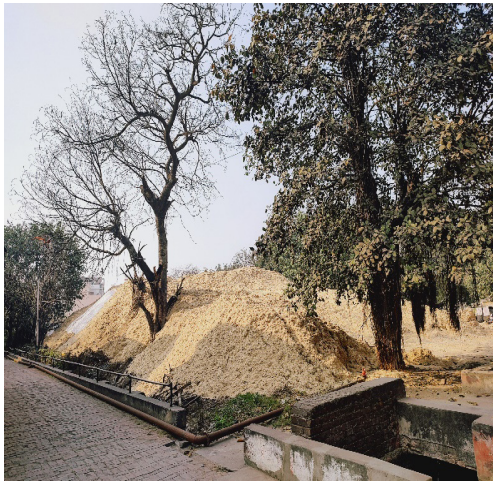
Bagasse storage in loose form to be used in boiler as fuel
