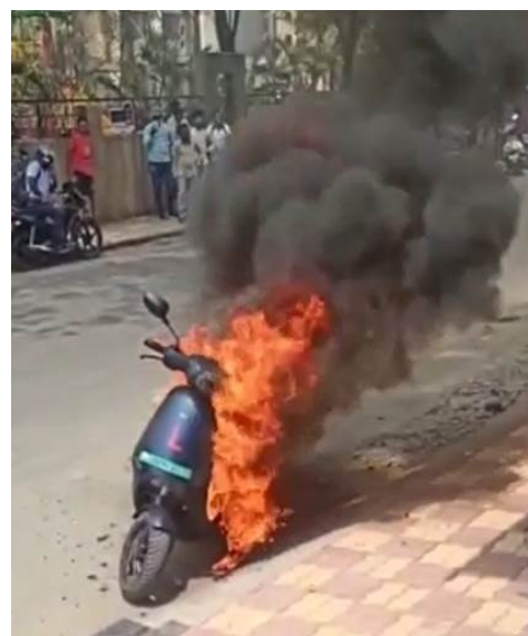
Figure 7: Electric two wheeler on fire due to thermal runaway of the battery
