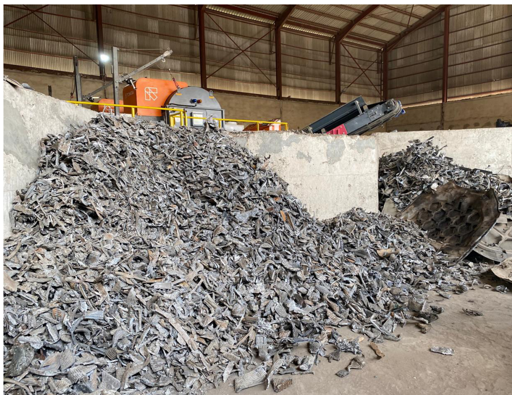
Shredded scrap waste to feed in furnace
