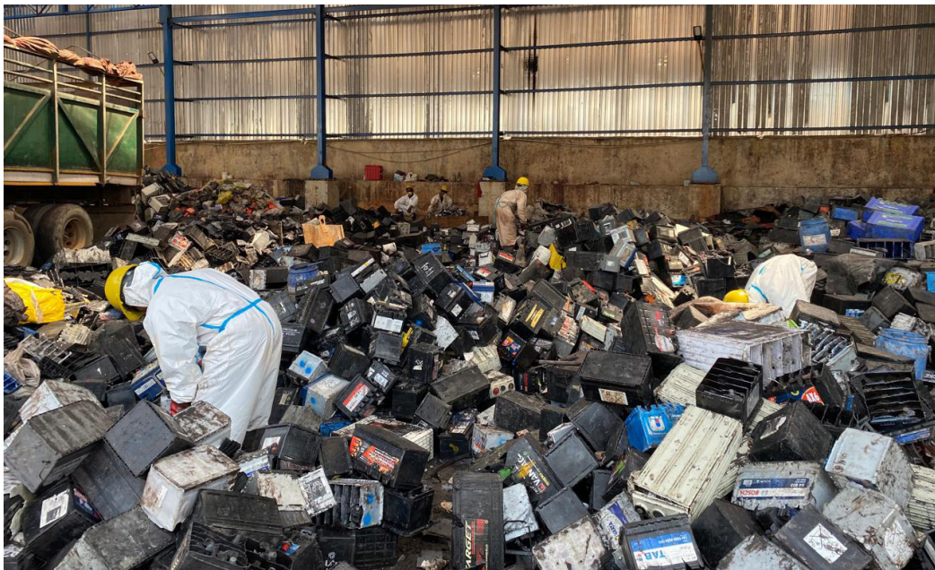
Manual dismantling of waste batteries at Hanushi Manufacturing
