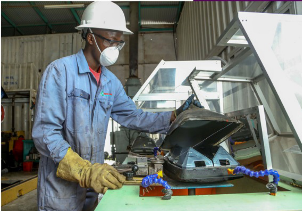
Dismantling of cathode ray tube monitors at Waste Electrical and Electronic Equipment (WEEE)
