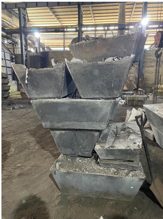
Moulded lead blocks made from scrap at Hanushi Manufacturing
