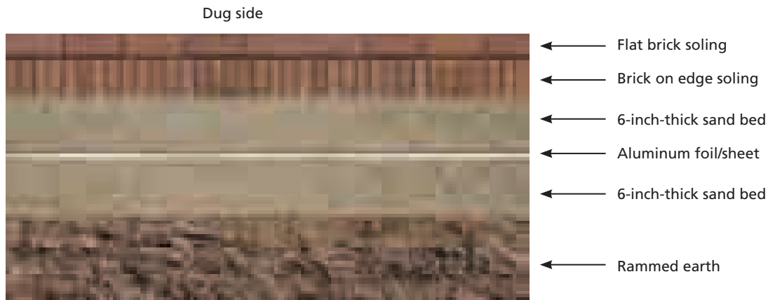
Figure 18: Kiln floor design
