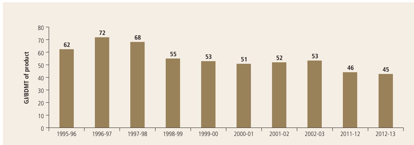
Graph 11: Energy consumption – very little has changed in the mills through the years
