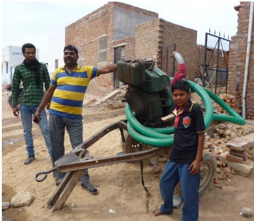
Figure 7: Generator based suction pump (Source: Rahul/CSE, 2015)
