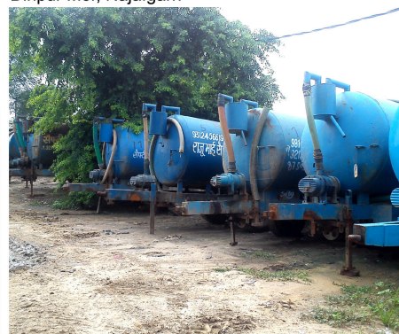
Figure 5: Tractor mounted vacuum tanker (Source Anil/CSE, 2015)
