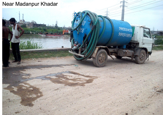
Septage disposal into Agra canal
