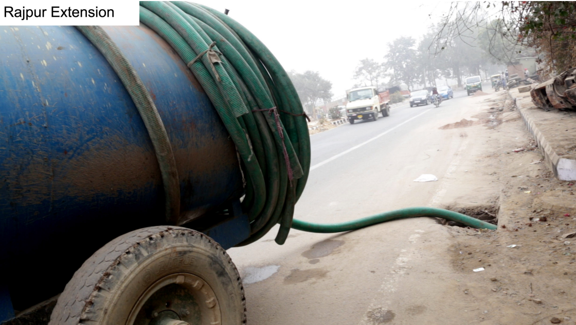
Septage disposal into storm water drain
