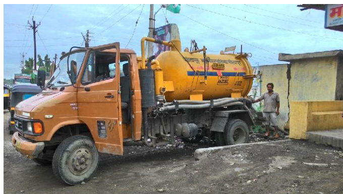
Figure 2: Vacuum tanker emptying septage from community toilet (Source: Rahul/CSE, 2015)
