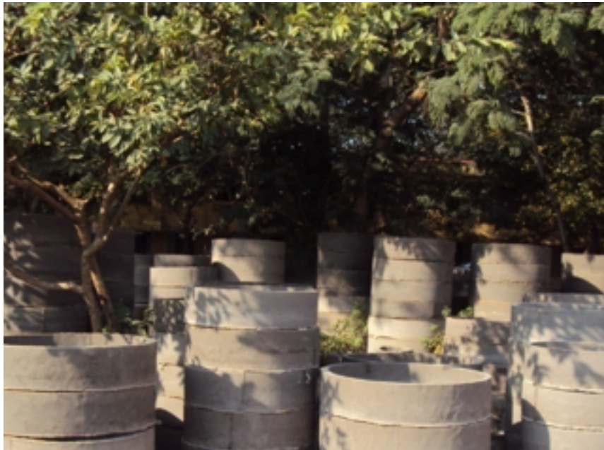
Figure 2: Prefabricated pits (Source Rahul/CSE 2015)
