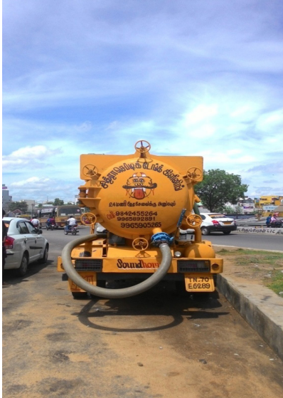
Figure 3: Vacuum tankers used for emptying onsite sanitation systems (Source: Bhitush, Rahul/CSE, 2015)
