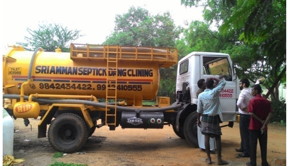
Figure 3: Vacuum tankers used for emptying onsite sanitation systems (Source: Bhitush, Rahul/CSE, 2015)
