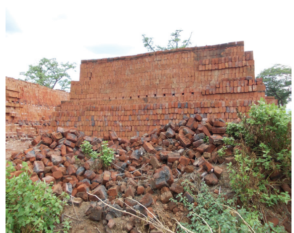
Over-burnt bricks as waste
