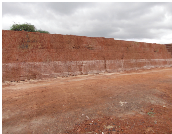
A large-scale clamp. Typically, they produce between 5–10 lakh bricks per batch
