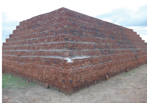
A large-scale clamp. Typically, they produce between 5–10 lakh bricks per batch
