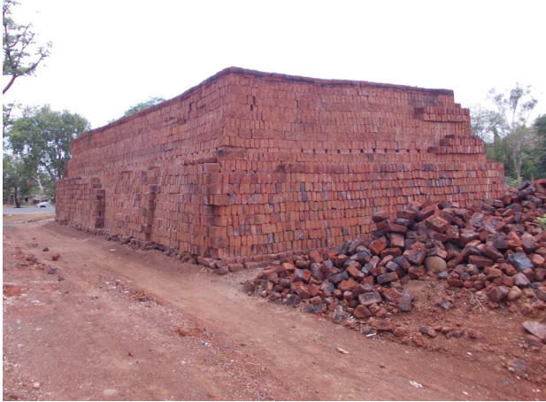
A clamp next to a road in Khopoli
