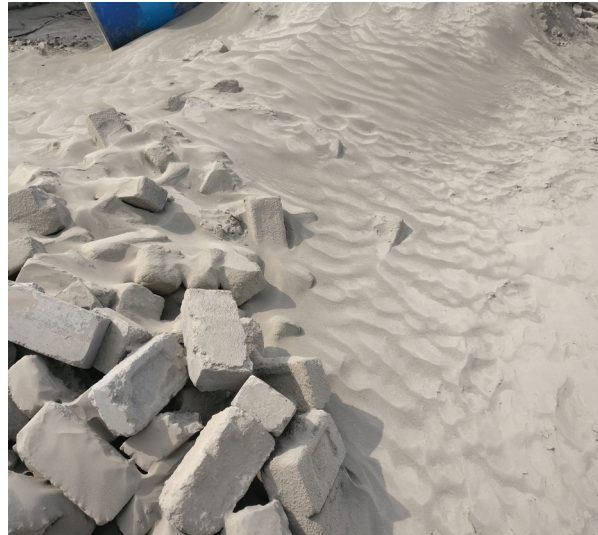
Ultra fine dry fly ash stored in open at a unit in Jhajjar
