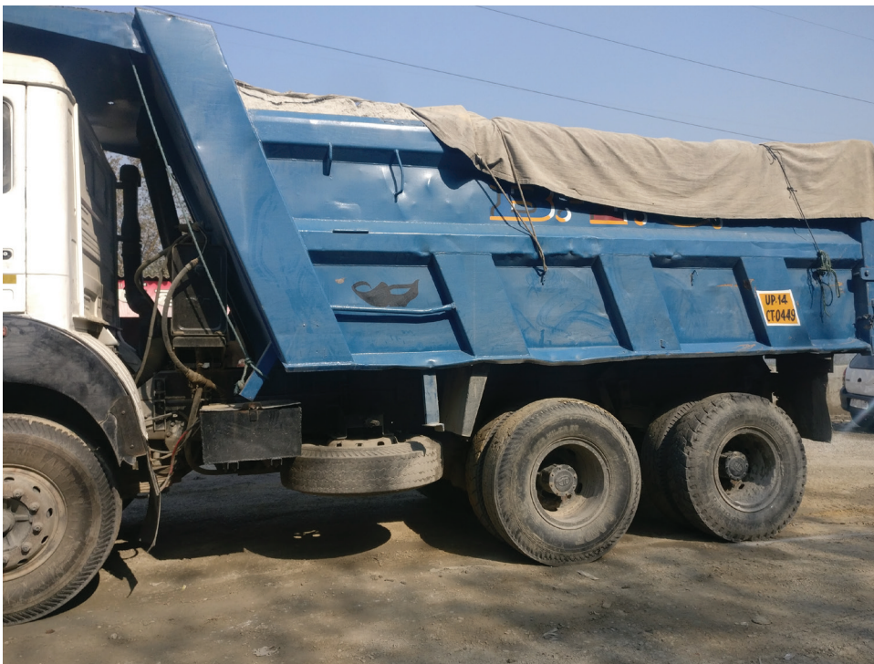
Hyva's covered with tarpaulin used to transport bottom/pond ash.
