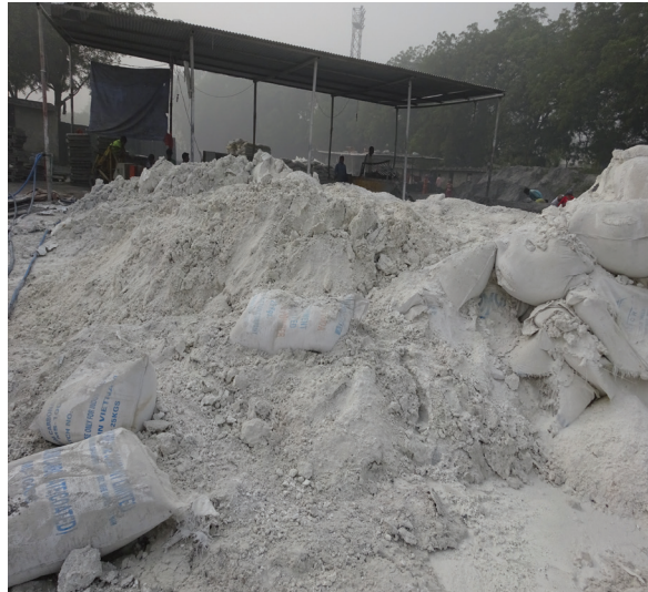
Torn lime bags due to hydration at a cluster in Nangli Sakrawati, Delhi
