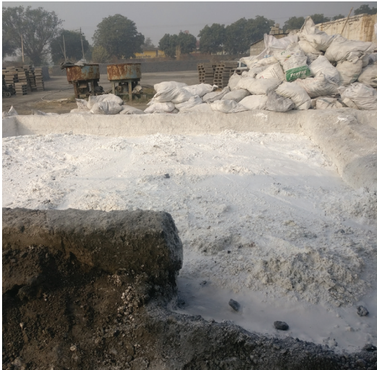
Pit designed for lime hydration in a unit at Gurugram
