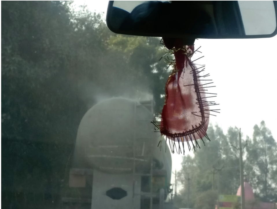
Fugitive emissions from Bulker carrying fly ash
