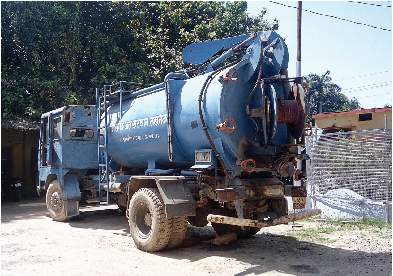
Suction cum sewer jetting machine
