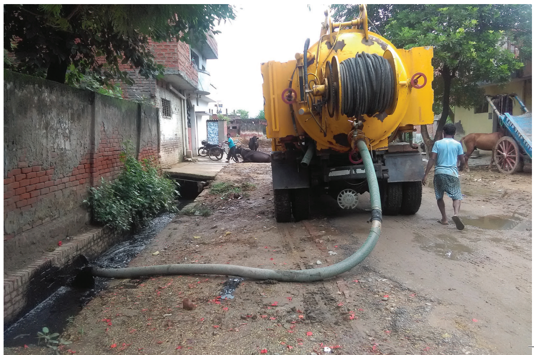
Faecal sludge discharged in open drain
