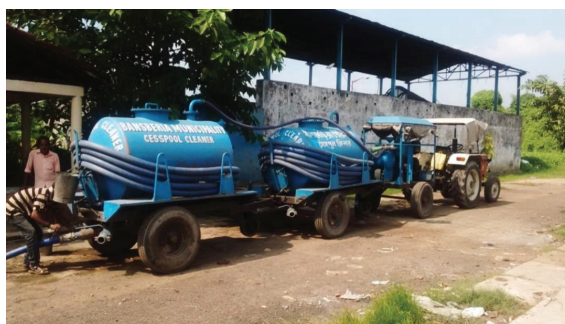
Figure 5: Tractor mounted vacuum tanker (Source: Anil/CSE, 2016)
