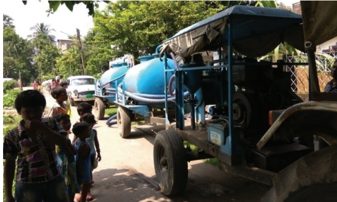
Figure 6: Suction pump of 5HP assembled with the tanker (Source: Anil/CSE, 2016)
