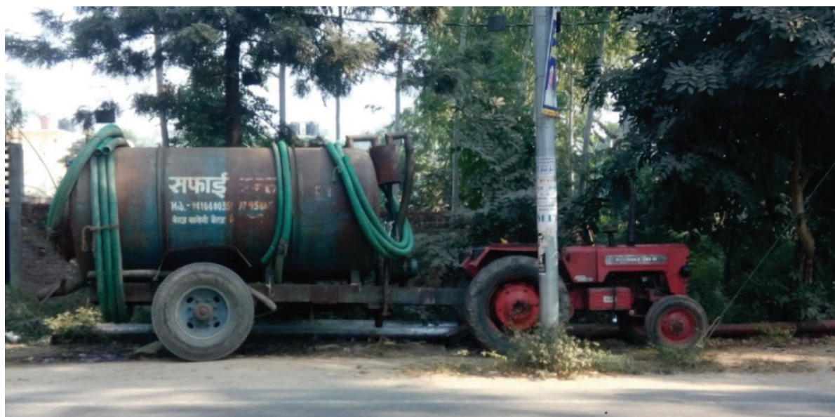
Figure 5: Vacuum tanker (4,000 litres capacity) used for emptying of OSS (Source: Amrita/CSE, 2016)
