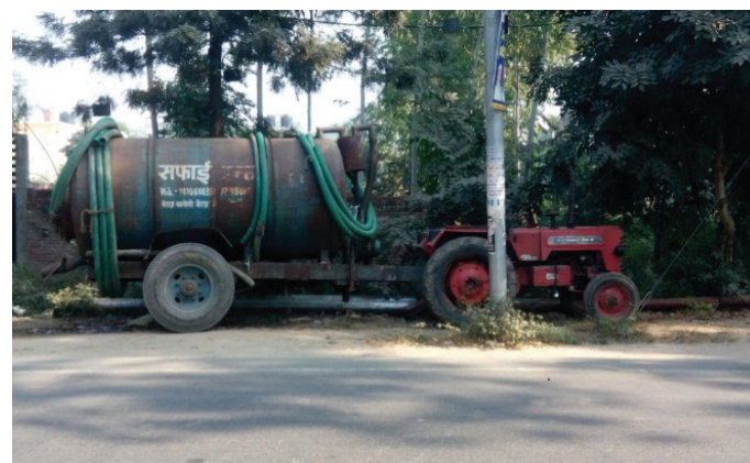
Figure 3: Vacuum tanker (5,000 litres capacity) used for emptying of OSS (Source: Amrita/CSE, 2016)
