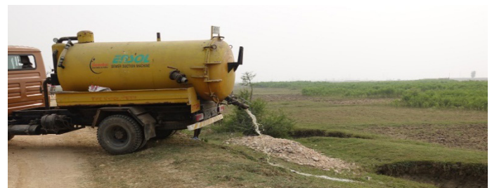
Figure 3: Septage being discharged into open fields (Source: Aishwarya/ CSE, 2016)
