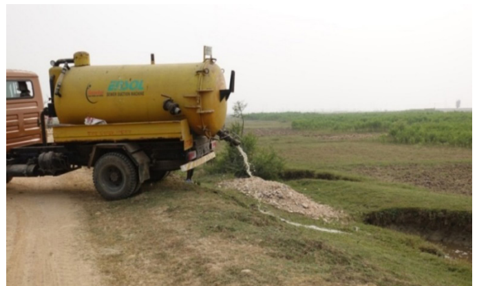
Figure 7: Septage getting emptied into open field (Source: Aishwarya/CSE, 2016)
