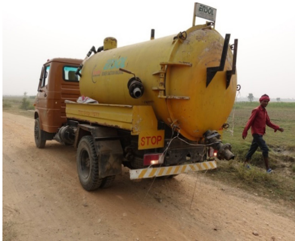
Figure 6: Truck mounted vacuum tanker (Source: Aishwarya/CSE, 2016)
