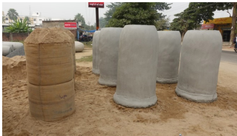
Figure 3: Prefabricated tank - locally known as septic tank (Source: Aishwarya/CSE, 2016)
