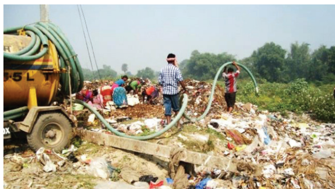
Figure 1: Discharge of faecal sludge at solid waste disposal site (Source: Anil/CSE, 2016)
