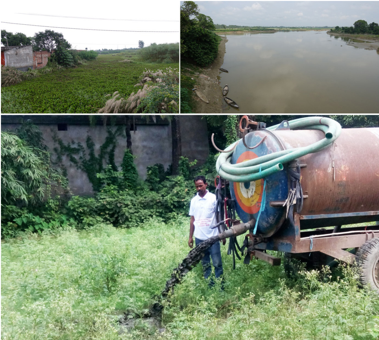
Figure 8: Discharge of FS in open fields by ULB vacuum tanker (Source: Anil/CSE, 2016)
