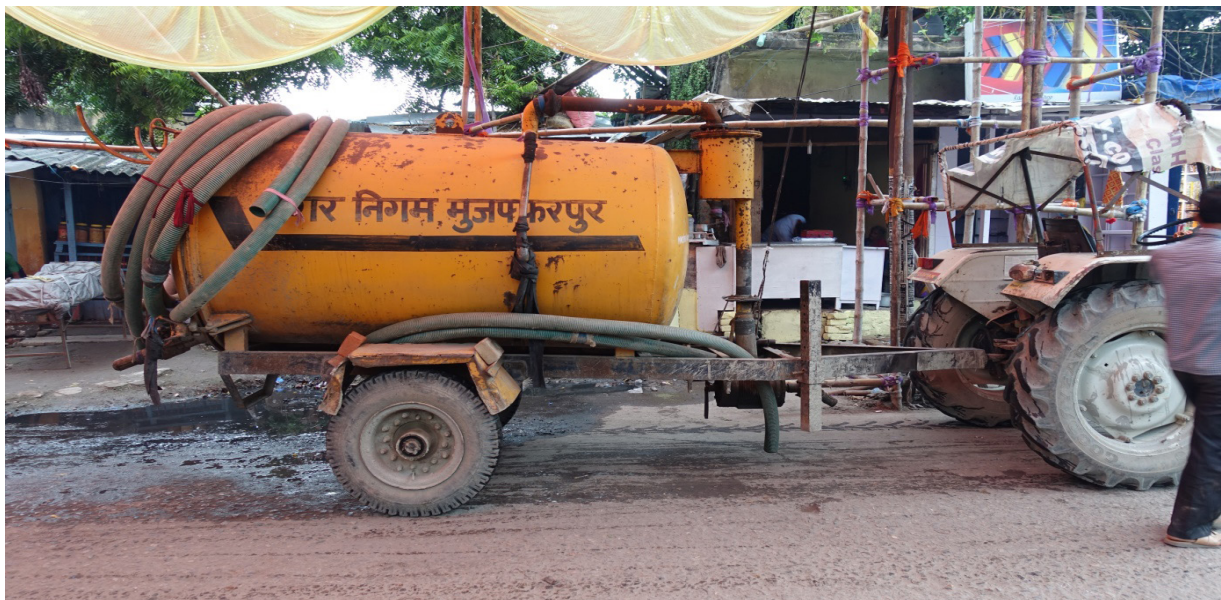
Figure 6: Tractor mounted tanker used for emptying service (Source: Amrita/CSE, 2016)
