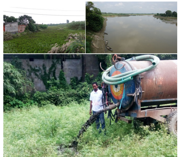
Figure 1: Discharging of FS in open fields
