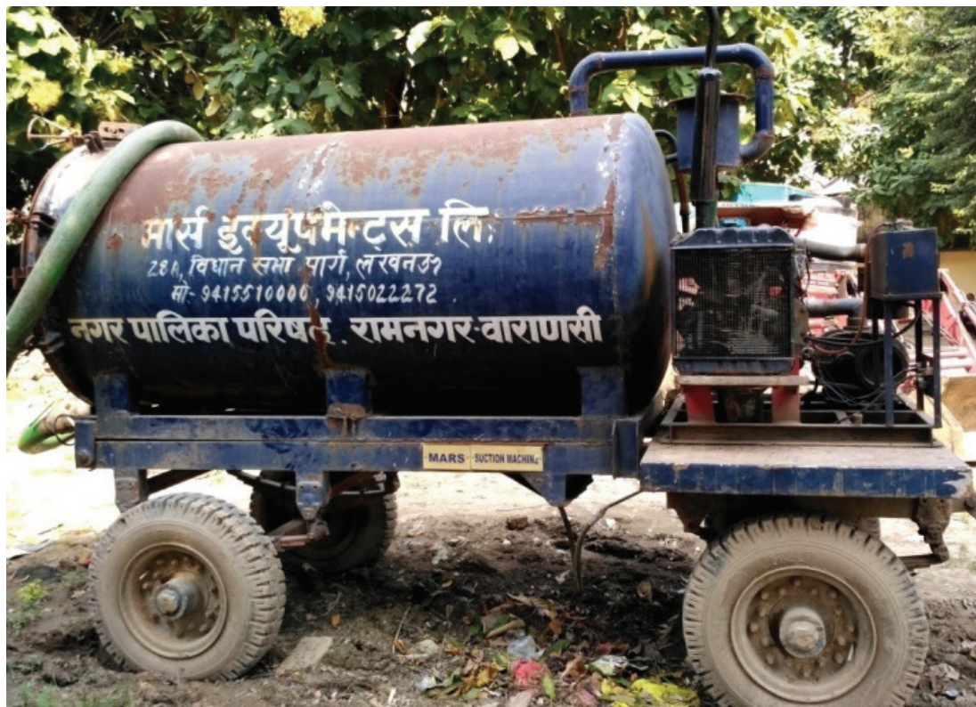
Figure 4: RNPP vacuum tanker used for emptying septic tanks/pits (Source: Shantanu/CSE, 2016)
