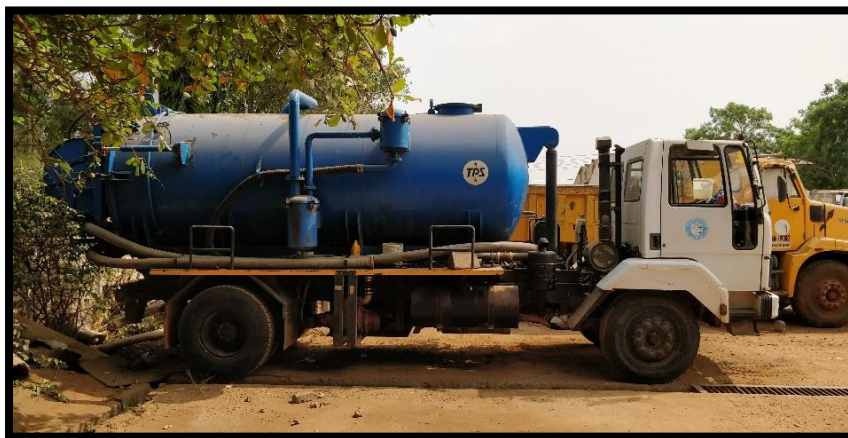
Figure 6: Vacuum tanker cum sewer jetting machine owned by WMD (Amrita/CSE, 2018)
