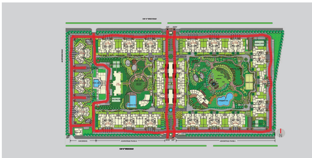
Figure 12: Marking thick lines over the roads on the site plan where cars are allowed can substantiate the data.
