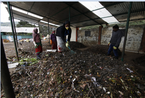
Composting of faecal sludge and organic waste in Nilgiri District
